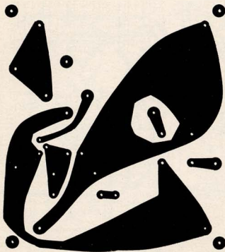
Fig. 6. Actual-size foil pattern for power supply. Like all the other PC boards, this one is also available etched and drilled (see Parts List for ordering details).
