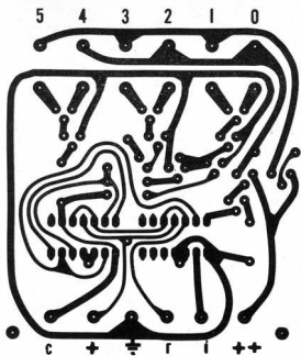
Fig. 2. Actual-size foil pattern for the modulo-six counter. It is the same size as the boards used for the other circuits (see text) simplifying construction of timer.
