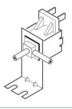
When de-energized, that straight front pipe connects to a filtered vent to ambient out the rear. When 12 volts is applied, those two front pipes are connected together and the ambient vent is blocked. While intended for vacuum uses, you can apply positive pressures on up into the 10 PSI range without any cracking problems. Yes, liquids can also be handled simply by glopping over the vent. Especially as an automated barkeep.
