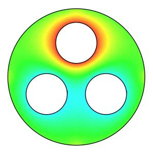
What we have here is a conduit with a triplet of three phase power lines in it. The top phase is shown at peak positive amplitude, while the bottom two will be at **one-half** their peak negative value. The outside shield is at ground potential.
