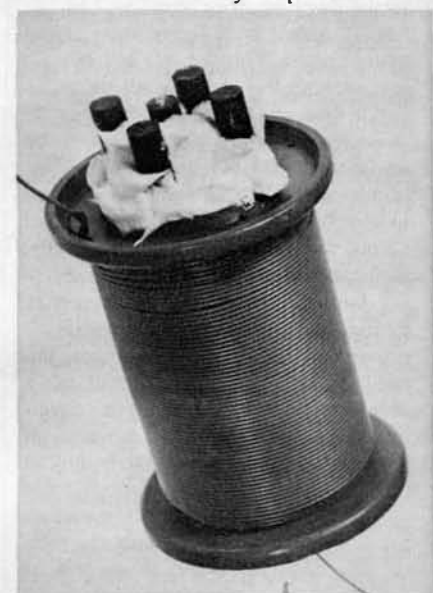
EXPERIMENTAL SUPER-LOOPSTICK is shown less shield. Rods are 5/16-inch long. Figure of merit is around 2. Resonating capacitor is around 235 pF.
