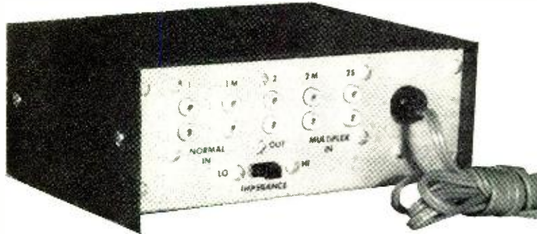
Rear view showing interconnecting jacks and impedance switch.
