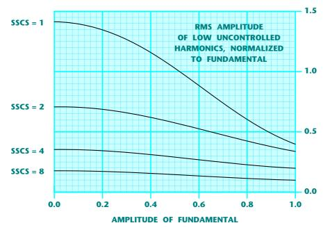
Another obvious benefit from spectrum spreading is that the filtering used should end up a lot more independent of amplitude. Thus further easing the filter needs.
