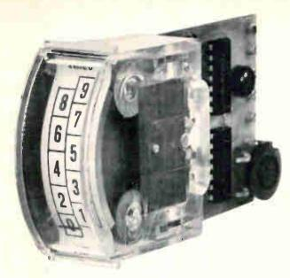
**\$10 per decade**. Digital displays built with milliammeter or incandescent bulbs and RTL circuits. In-line decades are easier to read and look better but meter version costs less and consumes less power.
