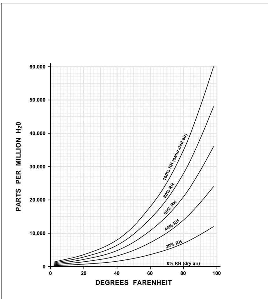
Fig. 1 – THE ALLOWABLE AMOUNT OF WATER VAPOR in air is a very strong function of temperature. Absolute humidity is a direct measure of that amount, expressed in parts per million or similar units. Relative humidity is instead a percentage ratio of how much moisture really is present compared against the maximum allowed for the current temperature.
