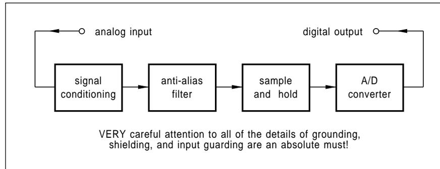
Fig. 1 – An analog to digital conversion system normally will need all of the areas shown here. Often, the A/D converter chip itself will be the least of your worries.
