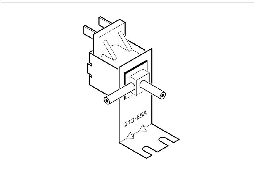
Fig. 1 - 3-Way automotive TCS valves are available surplus for as little as thirty cents each! They are ideal for robotics and for most other low pressure pneumatic hacking applications.
