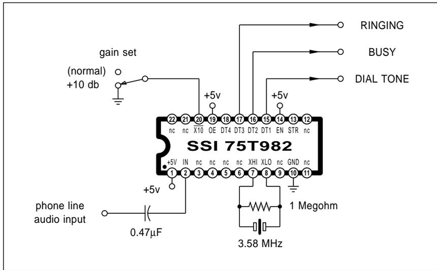
Fig. 2 – A CIRCUIT TO DETECT the "new" or "precise" call progress signals. This is a Silicon Systems chip; others are available from Signetics or Teltone.
