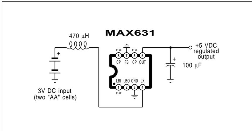
Fig. 4 – This simple switching regulator steps up two AA cells to give you a fixed +5 volt output at 10 Milliamperes. A pass transistor can be added for more output current.
