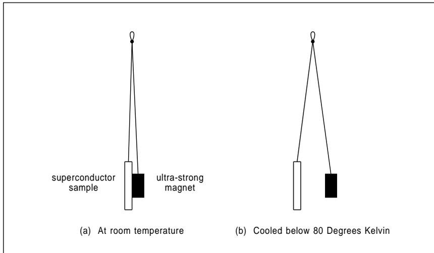
Fig. 2 – The Meissner Effect will produce a zero internal magnetic field in a cooled superconductor. The resulting field distortion will deflect (or can even levitate!) an extremely strong magnet as shown.
