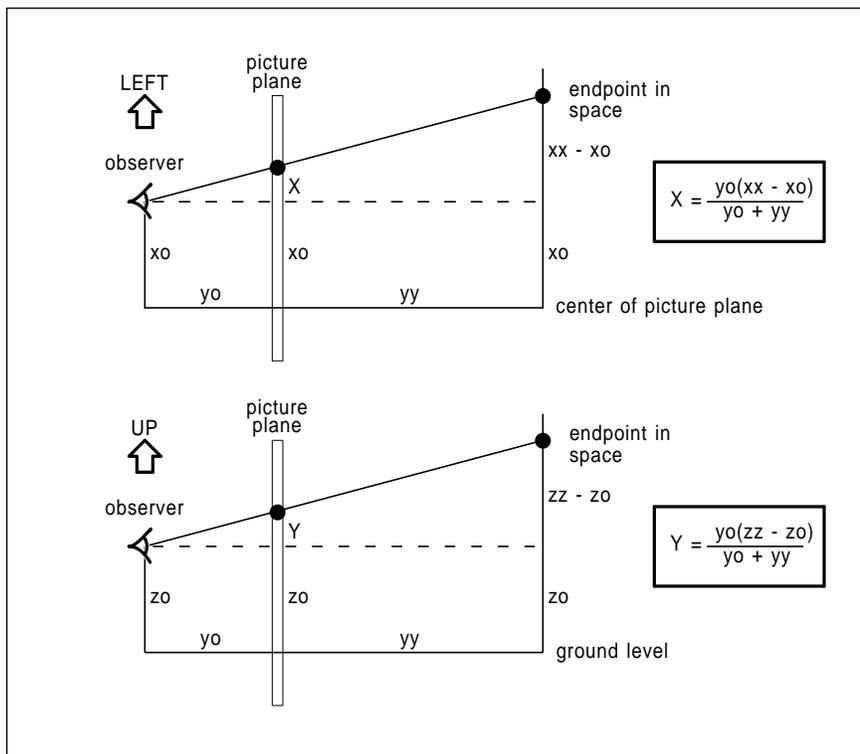
Fig. 6 – The 2-point perspective X and Y transforms. These can be easily included in a BASIC, "C", PostScript, or machine language program.
