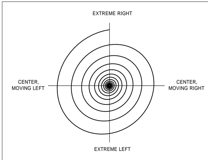
Fig. 5 – The phase plane plot of a damped pendulum. Phase plane plots do have important uses in response curves, system stability, chaos theory, and for many unusual artistic effects. Note that time is a parameter that advances inward along the path of the phase plane plot.
