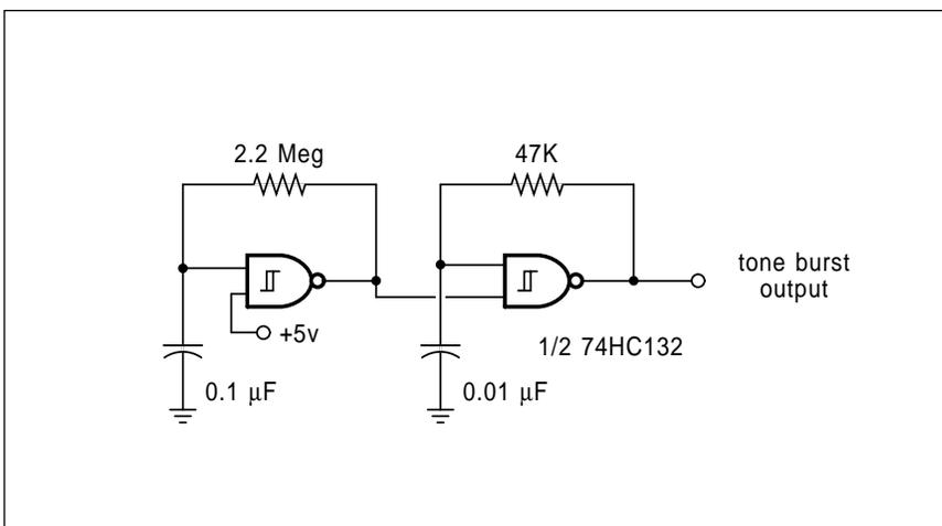
Fig. 3 – A GATED OSCILLATOR produces repeated tone bursts. The right RC values set the frequency, while the left ones determine the repeat rate.
