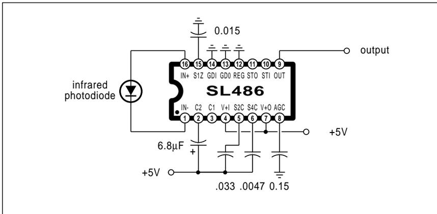
Fig. 2 – An infrared remote control preamplifier is usually needed between your receiving photodiode and the final digital decoder circuitry.
