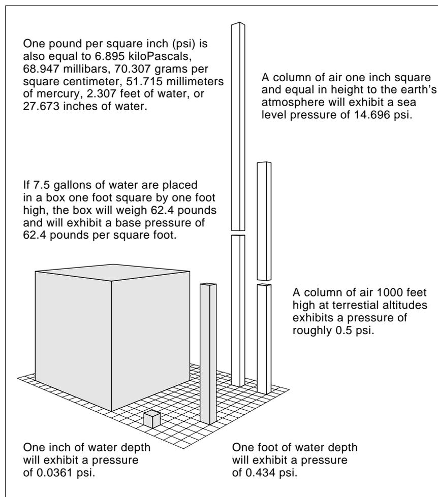
Fig. 1 – Here are some of the fundamentals behind pressure measurement.
