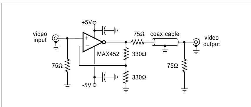
Fig. 4 – The video driver is separately available as the MAX452.
