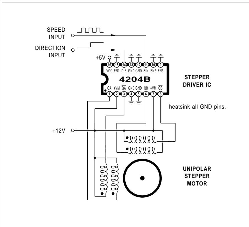
Fig. 5 – LOW COST SINGLE-CHIP stepper motor drivers are readily available from Motorola, SGS, and Sprague. Here is a popular and very low cost Sprague driver circuit.
