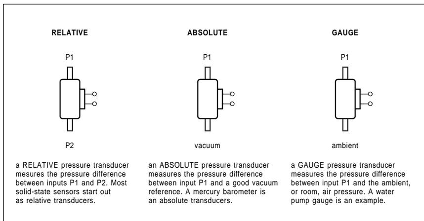
Fig. 2 – There are three fundamentally different types of pressure sensors. Most of the new solid state transducers start out as relative devices.
