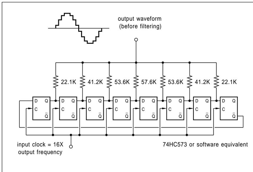
Fig. 5 – A sixteen step digital sinewave generator gives you an even better looking waveform. Here the fifteenth and seventeenth are the first harmonics present. That apparently "missing" resistor helps flatten out the waveshape.
