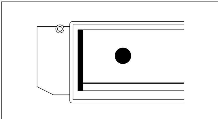
Fig. 1 – A Canon CX toner cartridge has to be modified before it can be refilled. First, remove the large cardboard label (not shown here) by lifting it up from each end. Then, drill a clean 1/2 inch hole in the fresh toner tank using a Vise Grip #3 Unibit. Carefully remove the chip.
