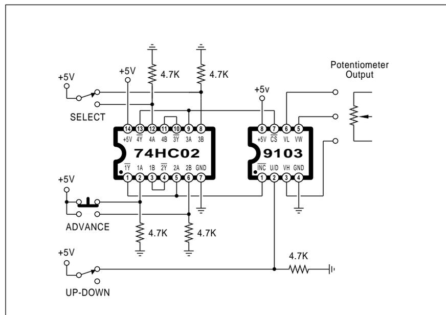
Fig. 3 – Use this circuit to test your EEPROM. The debouncing shown is only needed when you are using mechanical contacts.
