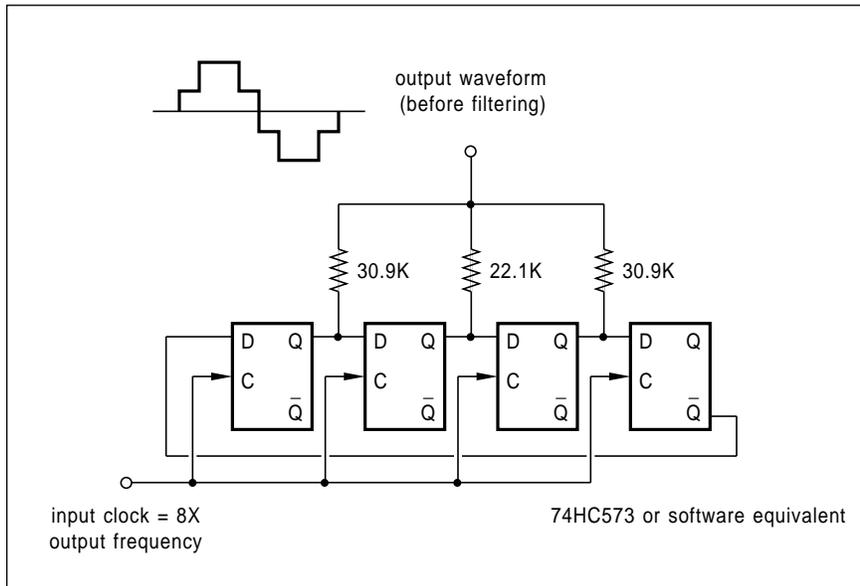
Fig. 4 – A Walking Ring digital sinewave generator of eight steps uses a "magic" waveform that has no low harmonics and thus is very easy to filter. The first harmonics are the seventh at one/seventh and the ninth at one/ninth of the fundamental amplitude.
