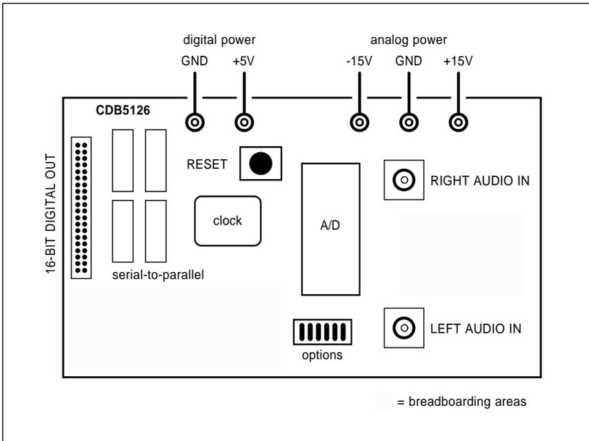
Fig. 3 – THE LAYOUT OF THE CDB5126 stereo audio front end. You literally squirt your stereo audio into the right side connectors, and 16-bit digital bits and bytes pour out the left. Note that digital +5 volt supply power must be applied AFTER the analog power or serious damage can result.
