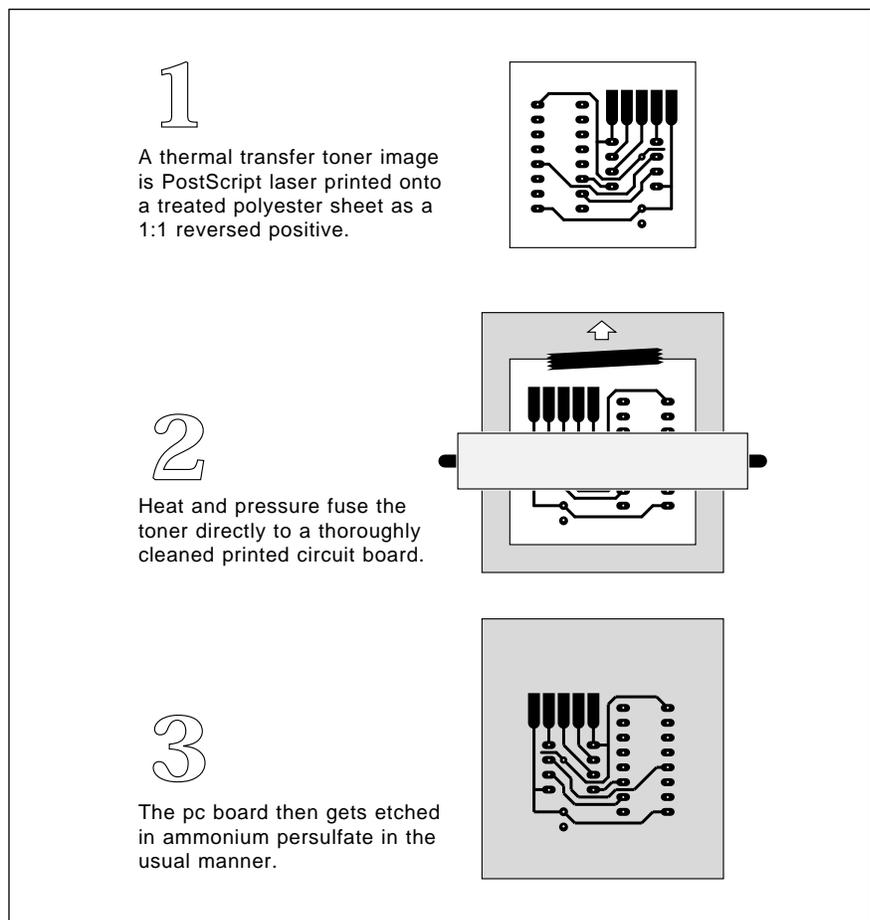
Fig. 3 – OUR NEW DIRECT TONER TRANSFER method can dramatically simplify and speed up making all of your hacker printed circuits at costs of only pennies per board. The process takes around twenty seconds.
