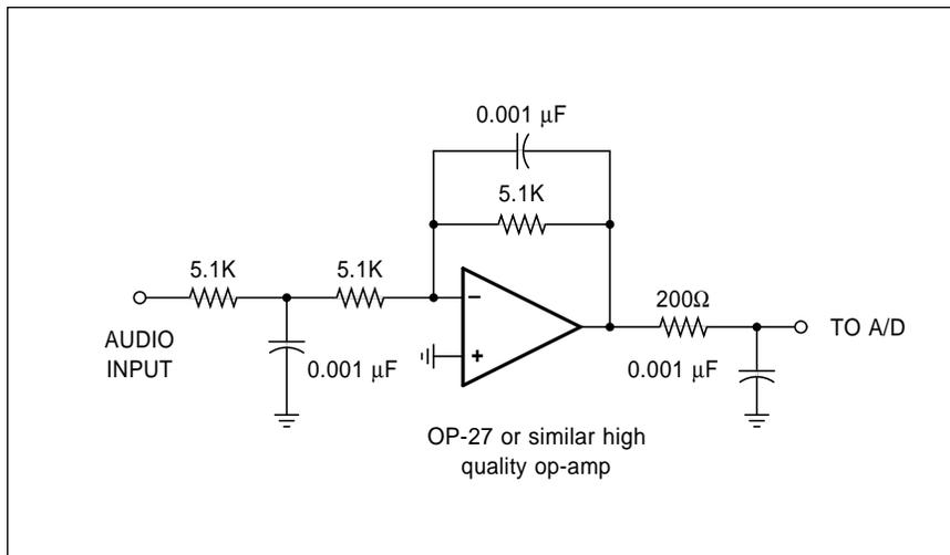
Fig. 4 – A RECOMMENDED INPUT DRIVER CIRCUIT. Additional anti-alias filtering is likely to be needed for your final CSZ5126 application.
