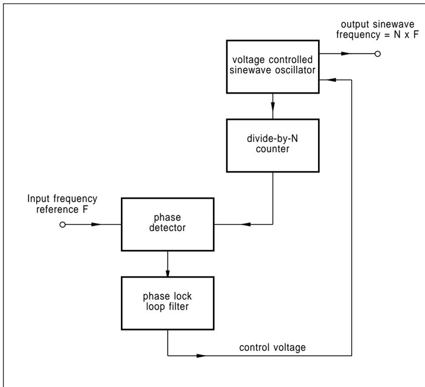
Fig. 2 – The phase lock loop can generate digital sinewaves and does get particularly useful where many different channels are desired for frequency synthesis. Changing "N" changes the channel selected.
