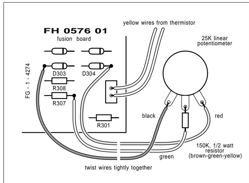
Fig. 6 – The pictorial diagram for the Canon fuser unit modification. The mod costs around 60 cents and can be done in twenty minutes.
