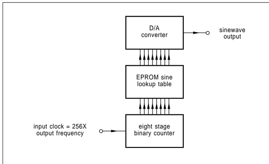
Fig. 3 – Table lookup of digital sinewaves gives a clean waveform and high accuracy, but is often limited to lower frequencies, especially when done by using personal computer software.
