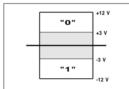
Fig. 2 – Here are the two logic levels that are normally needed for RS-232 communications. A "negative logic" convention is always used.
