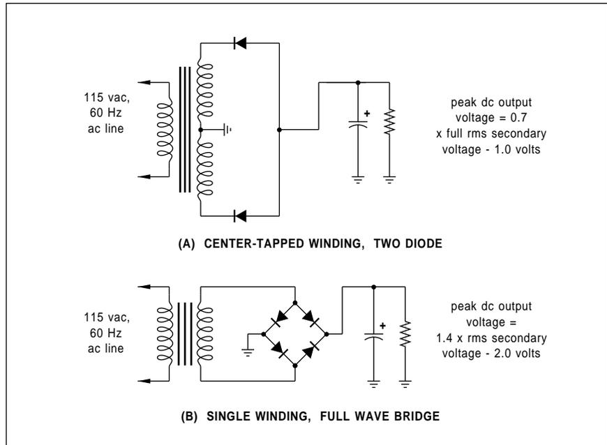
Fig. 1 – TYPICAL FULL WAVE LINE OPERATED "brute force" dc power supplies. Picking the correct value for a ripple filter capacitor turns out to be a lot easier than you might first suspect. The resistor represents a voltage regulator or other circuit load.
