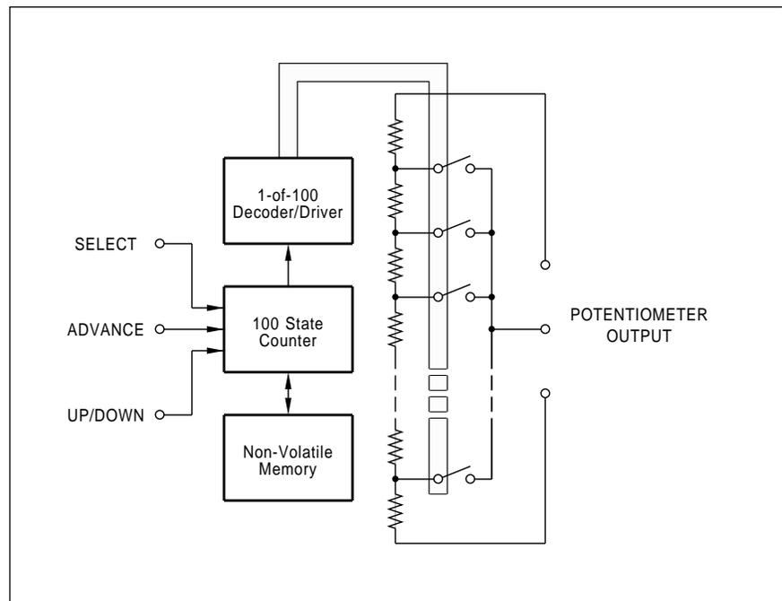
Fig. 1 - An EEPOT can simulate any ordinary potentiometer that might be remotely controlled, either manually or by a computer. The wiper position is remembered during unpowered times by an internal non-volatile memory.
