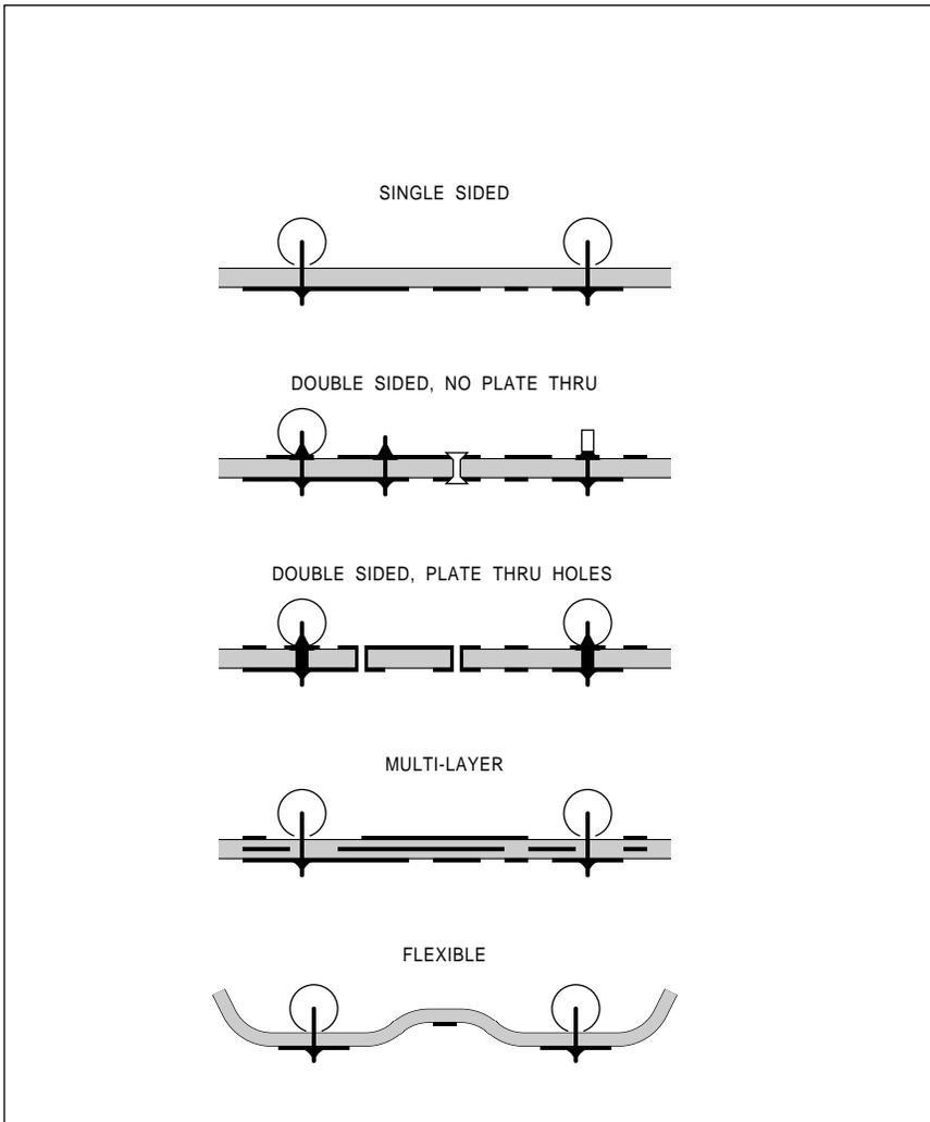
Fig. 1 – SEVERAL POPULAR TYPES of printed circuit boards. Note that a double sided plate thru board can be hacker faked by using component leads, eyelets, wire tabs, or low cost individual pin sockets.
