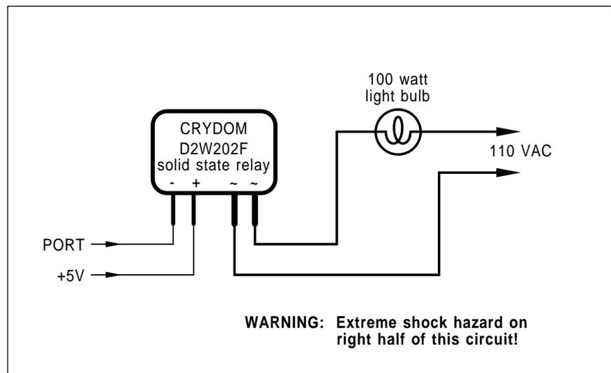
Fig. 2 – This simpler but more expensive ac power output computer interface needs only one part. Once again, a low logic input will light the lamp.
