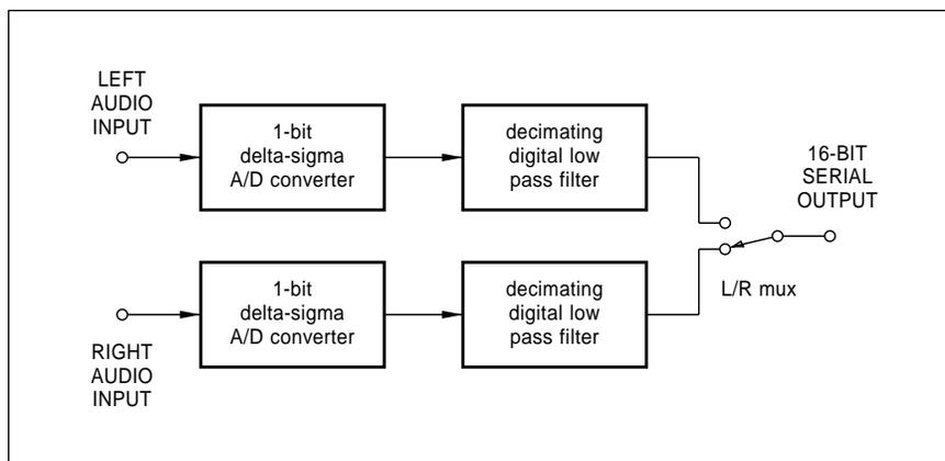
Fig. 7 – A SIMPLIFIED BLOCK DIAGRAM of the CSZ5326 A/D. The mind blowing specs here do include a 95 decibel dynamic range, 106 decibels of signal/noise ratio, 0.001 decibels of passband ripple, and a 0.0015 percent harmonic distortion for both 44 kHz stereo channels.
