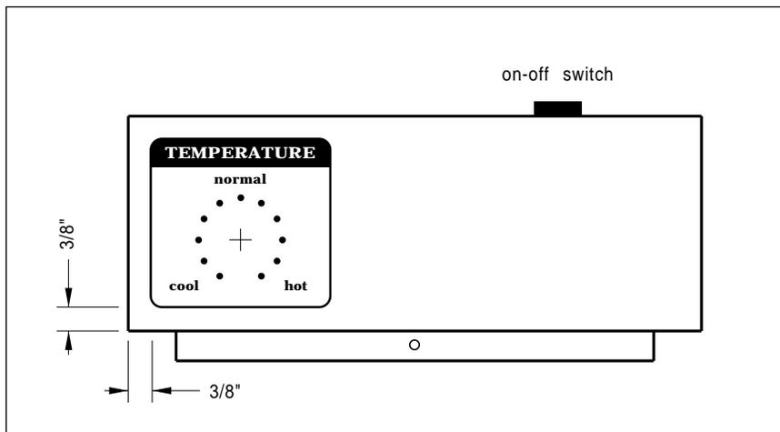
Fig. 5 – Position the decal exactly as shown here onto the front skirt of the right cover. A 13/32" hole is then drilled at the crosshairs.
