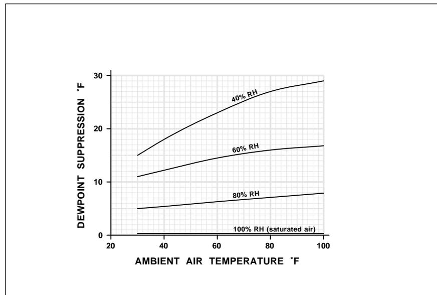
Fig. 3 – PRECISION LABORATORY MEASUREMENT of relative humidity is done by chilling the air to its dewpoint to find the equivalent air temperature for full saturation. Usually a servo driven mirror will fog or frost at the dewpoint, altering a sensing beam of light. Dewpoint measurements are best used at the higher humidity and temperature ranges.
