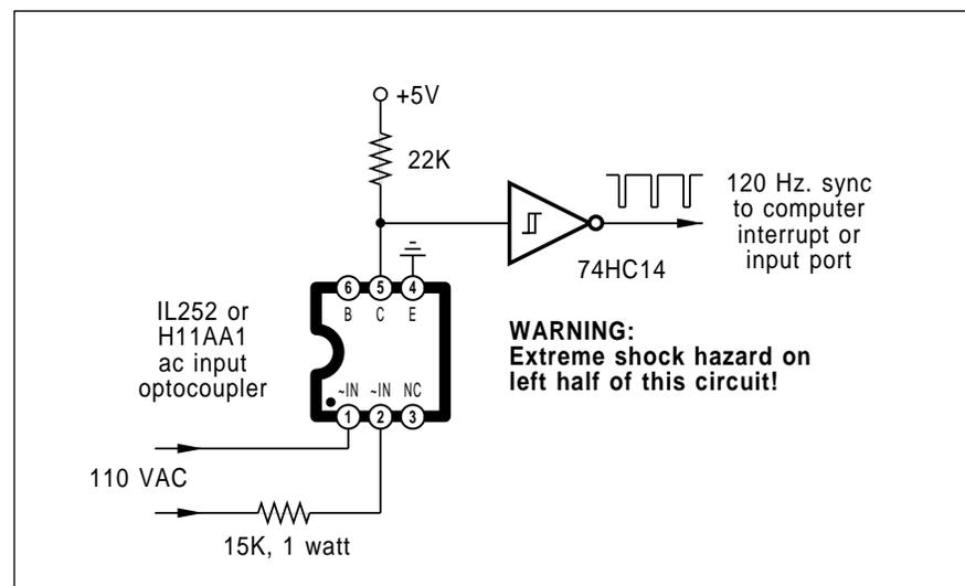
Fig. 4 – A line synchronizer input circuit is used to lock computer or controller phase timing to the ac power line. Note that this uses a special "ac input" optocoupler that lights with either input polarity.
