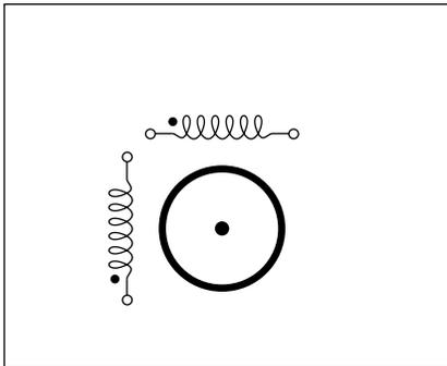
Fig. 1 – IN A BIPOLAR (or unifilar) stepper motor, there is only a single winding for each phase. Although the stepper itself is powerful and low in cost, the driver circuitry gets extra complicated since a full bridge circuit is required that is able to route current in either direction. Bipolar steppers often have four leads.
