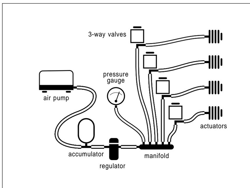
Fig. 3 – A typical low pressure air system. Note that three-way valves MUST be used; otherwise, the air will stay stuck in the tubing and all of the actuators will remain extended.
