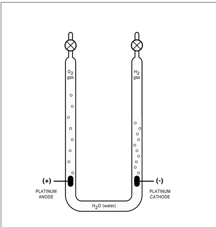
Fig. 1 – AN ELECTROLYTIC CELL is the key to the cold fusion experiments. This simple cell will break down or dissociate the water molecules into their hydrogen and oxygen atomic components.
