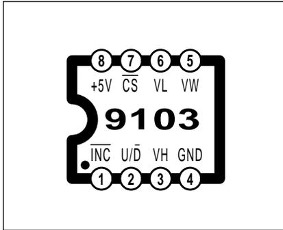
FIG. 2 – EEPTOT Pinouts. VL, VW, and VH are the terminals for the output potentiometer. The  $\overline{CS}$  chip select is brought low to change the wiper position, but is otherwise left at +5. The position gets changed by bringing  $\overline{INC}$  first low and then high again, with the direction set by the up-down pin U/D. A high on U/D will advance the position.
