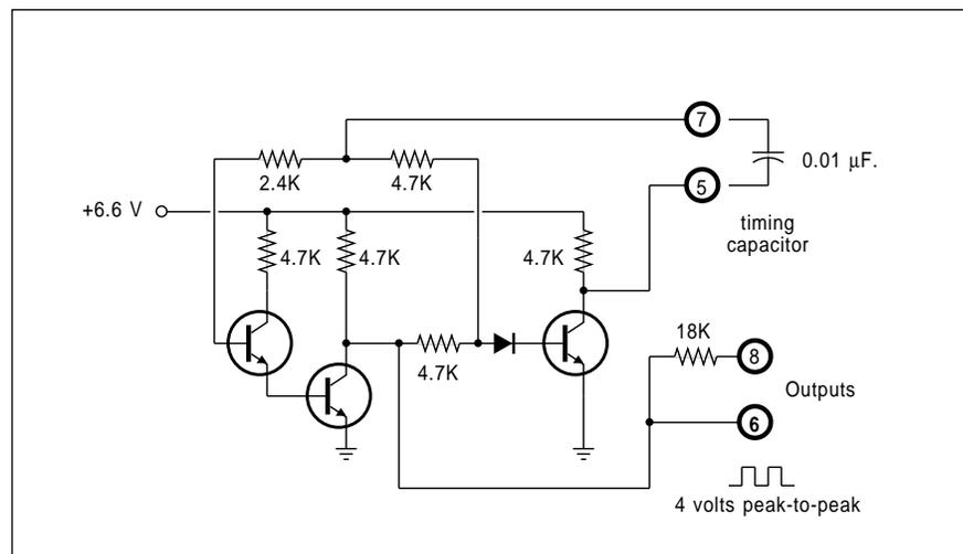
Fig. 4 – A simplified schematic of the internal audio oscillator found in the ULN 2429. The usual operating frequency is 2.5 kiloHertz, and can be set by the external timing capacitor.
