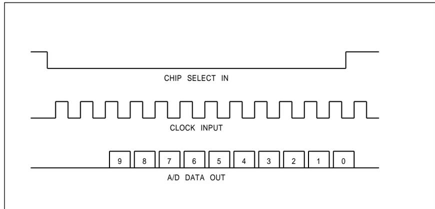
Fig. 4 – The timing waveforms used with the LTC1092. Your computer or other external timing inputs a chip select and thirteen clock pulses. Then, the LTC1092 responds in turn with ten A/D serial data bits. The A/D conversion speed can be as fast as 45 kHz.
