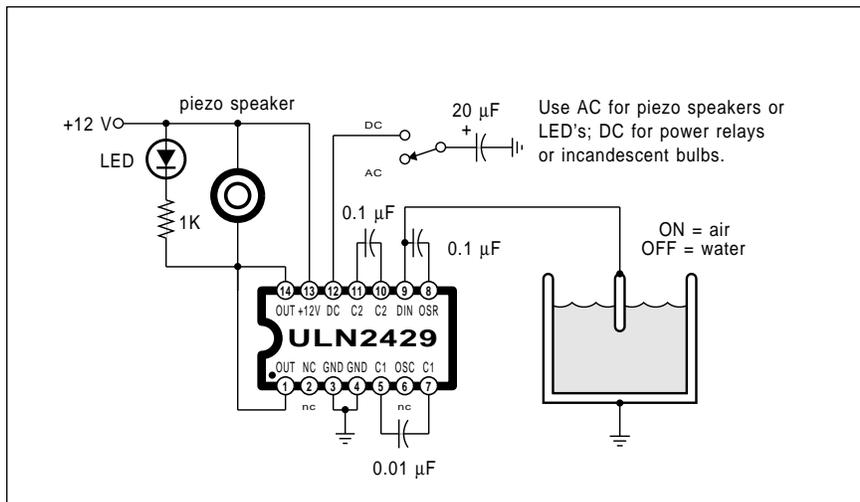
Fig. 3 – The Sprague ULN 2429 is an automotive liquid level detector that has plenty of hacker potential. Here is the basic test circuit using a pop can full of tap water as a liquid level sensor.
