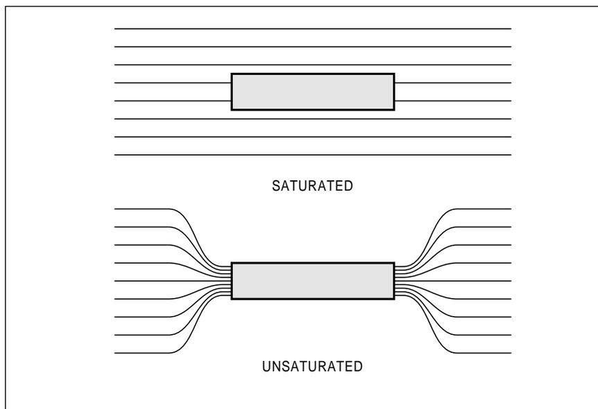
Fig. 1 – An unsaturated magnetic material will "pull in" the lines of force from the earth's or any other magnetic field. A saturated material will not.
