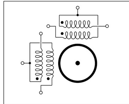
Fig. 2 – IN A UNIPOLAR (or bifilar) stepper motor, you will find a pair of windings for each phase. While this raises the cost and also reduces the available stepper power, your driver circuitry is vastly simpler and very much cheaper, since only a current sink is needed for each winding. A unipolar stepper often has six leads.
