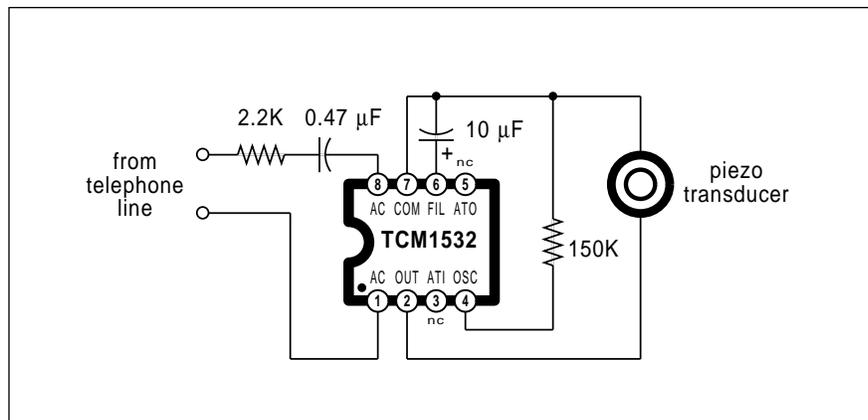
Fig. 5 – A combined ring detector and driver that directly powers a piezo transducer. Speakers or external amplifiers can be driven by transformer coupling. Note that all of the needed power is derived directly from the AC ring signal. Use a 400 volt input capacitor.
