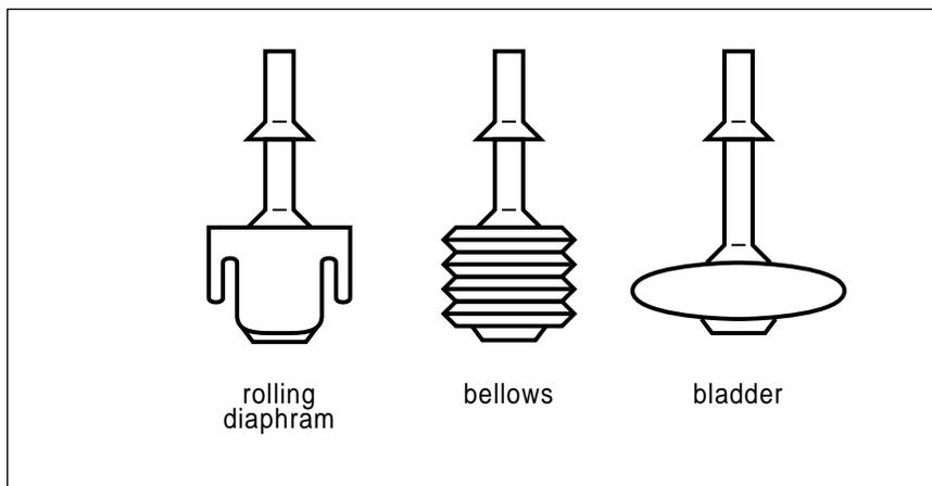
Fig. 2 – The foremost rule of low pressure hacker pneumatics is this: NEVER have any seal that moves! Here are some actuator ideas to get you started.
