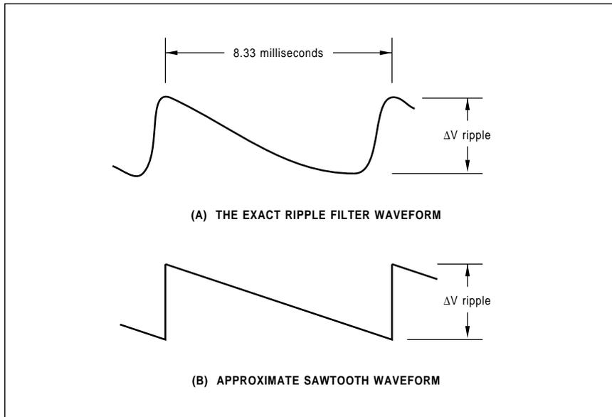
Fig. 2 – THE EXACT AND APPROXIMATE voltage waveforms as found across the ripple filter capacitor. Note that the diodes only conduct very briefly during the middle of each ac line half cycle.
