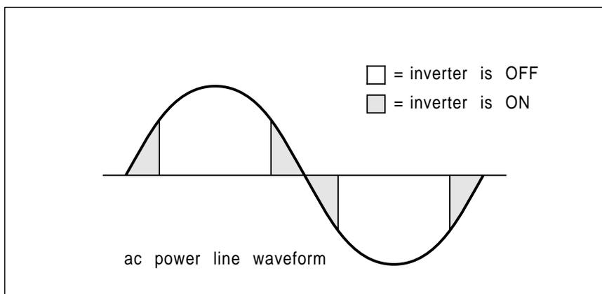
Fig. 6 – A synchronous inverter can be used to feed surplus energy from a solar panel or other alternate energy source back into the power line. Here is one possible waveform.
