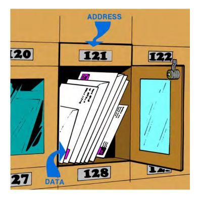
Repeating, an address is a location, and data is what goes in that location. Each address in a microcomputer has to be unique. No mixups are allowed. The addresses in the address space are often identified by a hex number. Typical working registers are usually identified by name or by a single letter.
