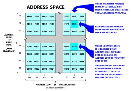
We see that we have 65536 boxes and that these boxes are numbered in order from hex \$0000 through \$FFFF. Besides finding a box by its number, we could also locate any box by finding its row and column instead.
