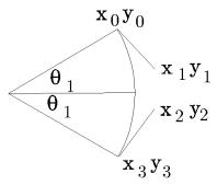
This arc is easy to model since it is symmetrical. We can see that  $x_0 = \cos(\theta_1)$ ,  $y_0 = -\sin(\theta_1)$ ,  $x_3 = \cos(\theta_1)$ ,  $y_3 = \sin(\theta_1)$ . Substitute these into the Bézier curve. So now the Bézier curve is less general and passes through the end points.
