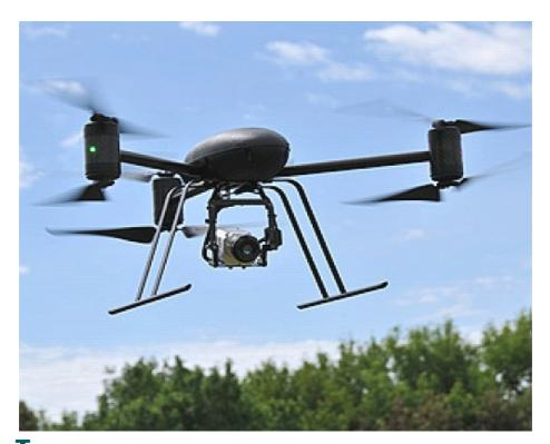
The Draganfly is a camera sized aerial drone and video capture system that should be eminently suited to further hanging canal exploration. Especially for finding non-obvious continuances.
