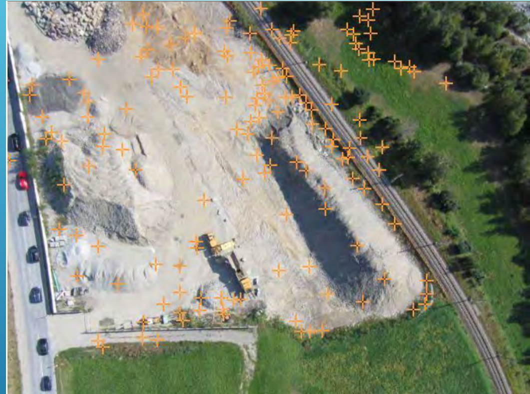
Figure 4. Automated tie points in a densified point cloud (Pix4D, 2022b)
