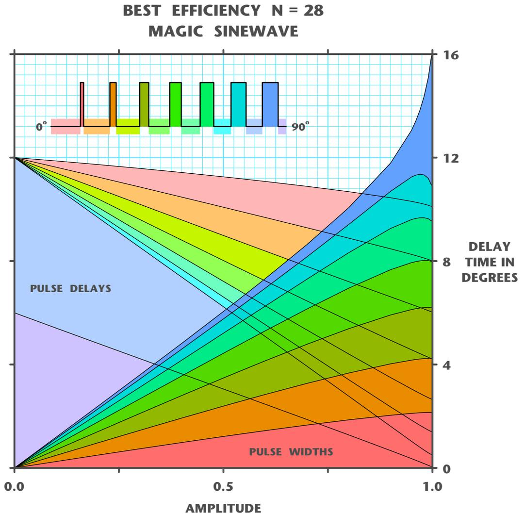
We can quickly tell that high amplitudes of **p7** will be the most critical. Owing to the "double whammy" of being both very large and very bent. You can use the **Magic Sinewave Calculators** to find how much worse the distortion gets with a pulse position or size error. Entering half a bit at 8-bit full scale 16 degree accuracy tells us that such a **p7** error here will only increase total distortion by a fraction of a percent.
