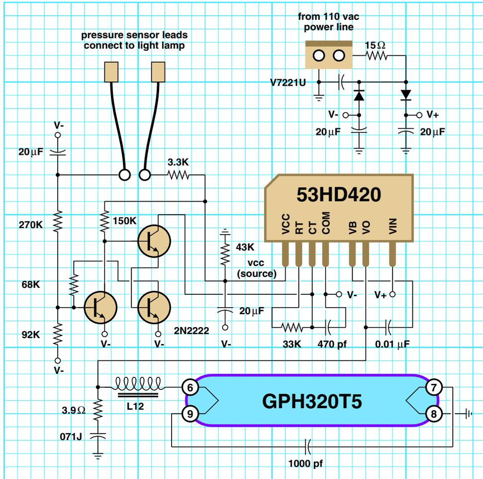
The heart of the circuit is the **International Rectifier** 53HD420. This converts a positive and negative line driven power supply into a 170 volt square wave at 34 kilohertz. This drives a serial RLC circuit consisting of the ballast inductor, the filaments of the lamp, and a resonating capacitor.
