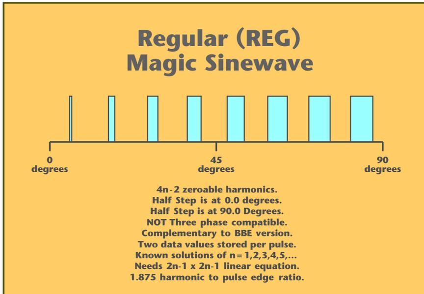
The REG Magic Sinewave has half steps at both 0 and 90 degrees. At first glance, it would not seem too useful in that **the BBE Magic Sinewave zeros out two more low frequency harmonics** "free" for the same number of pulses per quadrant.
