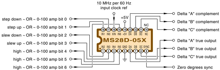
This delta friendly eval chip has been set up in a **dual use mode**. Binary input amplitudes of 0 thru 100 directly output their normalized respective amplitudes. Higher binary input codes allow **step up**, **step down**, **slew up**, and **slew down** operation. More details on this chip appear [here](#).
