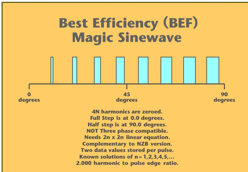
The first quadrant shown here will get mirrored and then flipped to form a full magic sinewave cycle. This guarantees **quarter wave symmetry** which in turn guarantees **no even harmonics** and **no cosine term odd harmonics**.
