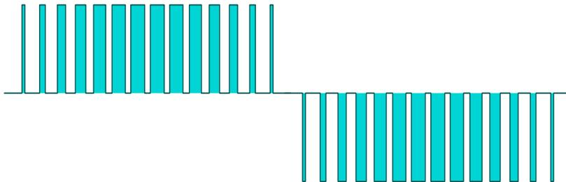
This can be viewed as a highly specialized form of **PWM** pulse width modulation. One that has **far fewer** transitions than normal for significantly higher switching
