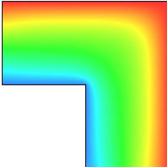
We can immediately see that the current density at the inside corner is **three or more times higher than normal!** And that this can cause excessive heating at higher current levels. Thus, all of those pretty square edges can easily cause you bunches of grief. To make your current density more uniform, do a 45 degree break at each corner, or use rounded edges instead.
