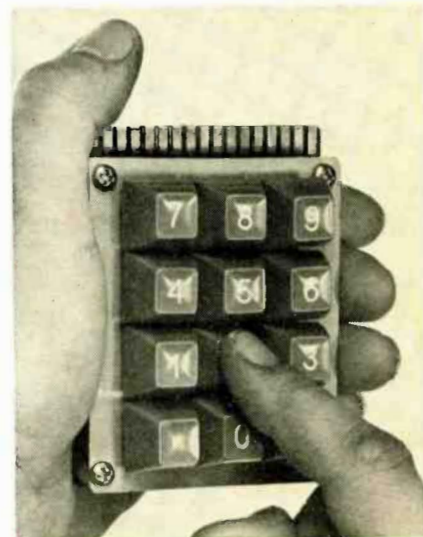
CALCULATOR KEYBOARD ready for mounting. Note the printed-circuit connector.
