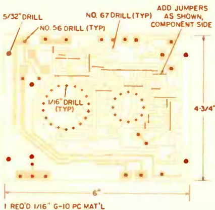
FIG. 3—PC BOARD MECHANICAL DETAILS. Drill as Indicated then install the jumpers.
