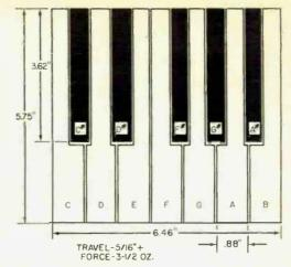
One octave of traditional piano or organ keyboard. White keys are different shapes in order to get a "piano" spacing in the front and even mechanical spacing at back.
