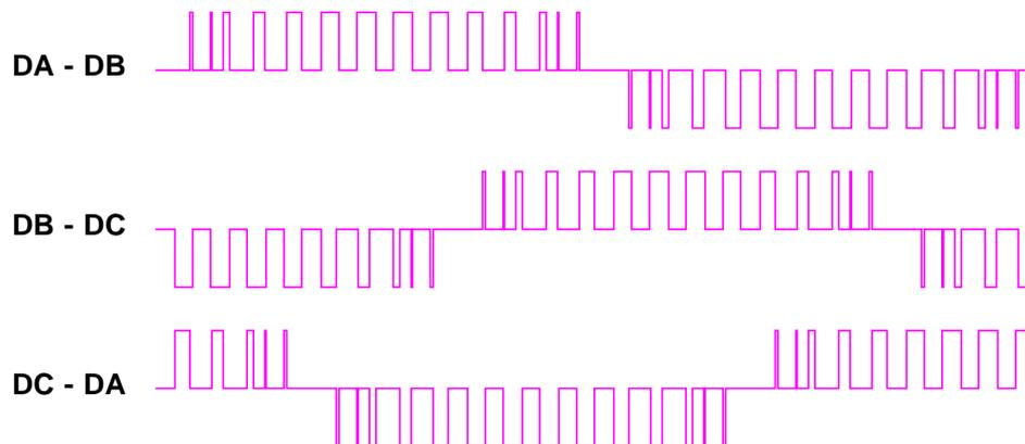
The bridge drivers will automatically take care of these subtractions for you. You also can **digitally subtract by ADDING one complement**. Which is quite handy to generate these bipolar analog test outputs...
