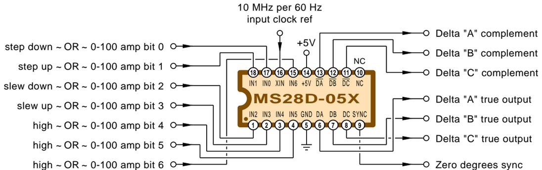
The 18 pin **DIP** chip is powered from a conventional +5 volt dc source and draws less than ten milliamperes. An external clock input reference of approximately **six Hertz per Megahertz** is required to set your output speed or frequency. A **ten MegaHertz** reference input thus becomes a **sixty Hertz** output frequency.
