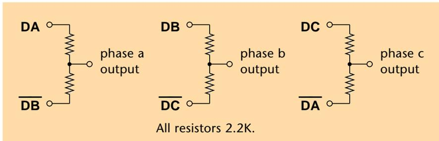
You can use similar resistive adding with opamps or filters. If not already provided, add a series 100 microfarad output coupling capacitor to block the 2.5 volt dc offset. Loading the ac output with a 1K resistor to ground will drop the output values to about a 0 DBM peak level.
