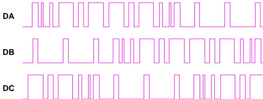
We see that the waveforms are forward and reverse symmetric. And are identical except for phase shifts of **120** and **240** degrees. These delta waveforms are derived [here](#), [here](#), and [here](#).
