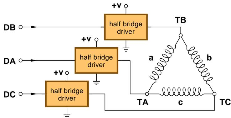
This assumes **non-inverting** half bridge drivers. Otherwise, the corresponding  **$\overline{DA}$** ,  **$\overline{DB}$** , and  **$\overline{DC}$**  lines are used. The half bridge supply voltage determines the **peak** of the output sinewave voltage for Amplitude 100. Minus on-state conduction drops.
