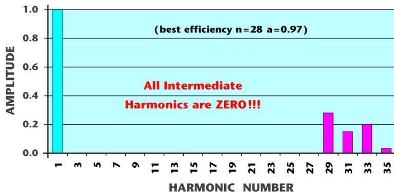
Although any chosen number of the **Magic Sinewave** lower harmonics could be forced exactly to zero in theory, the first two or higher **unsuppressed** harmonics will remain of significant size. These will typically range from **one fifth** the size of the fundamental for high amplitudes up to **matching** the size of the fundamental for very low amplitudes.
