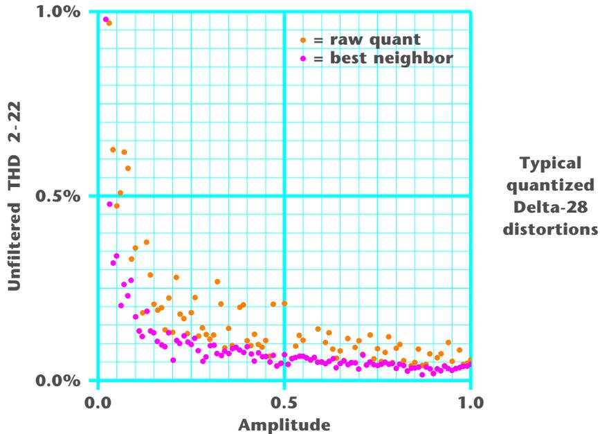
We see that our raw quantized total harmonic distortion for the second through twenty-second harmonic is under 0.2 percent for most higher amplitude values. And that is **before** any filtering. Our filter, of course, has bigger things to worry about. Namely the uncontrolled twenty third and higher harmonics.
