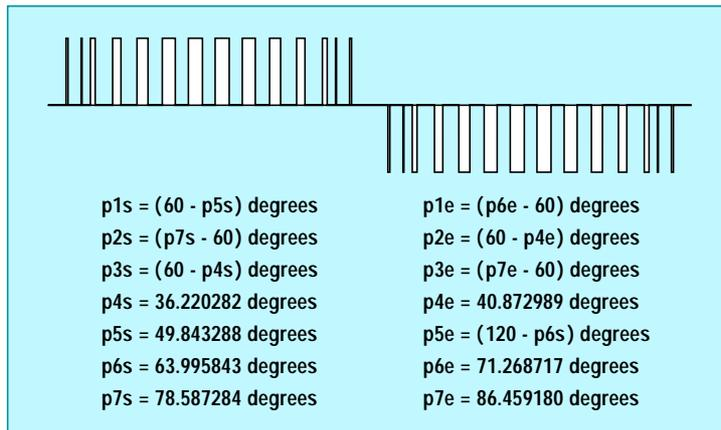
2. Three phase compatible "delta friendly" Magic Sine wave variant also has 0.53 amplitude. Even and odd harmonics 2-22 are zero. A mere seven table lookup values are needed per amplitude.
