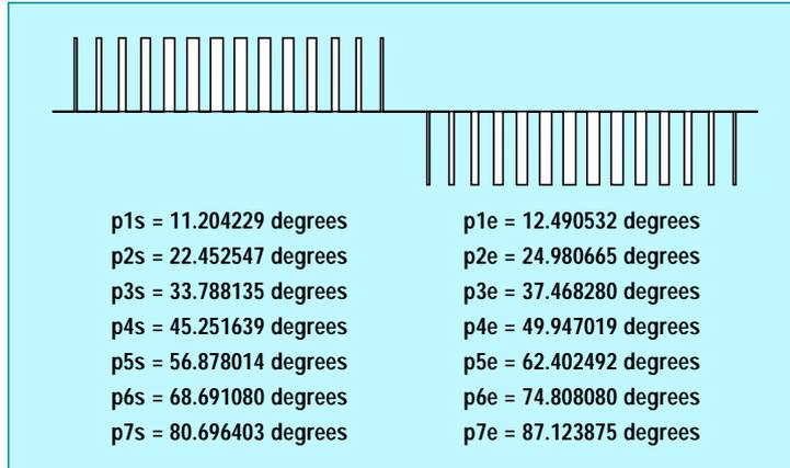
1. Seven pulse per quadrant steplocked magic sine wave offers an 0.53 amplitude and complete zeroing of all even and odd harmonics 2 through 28. Pulse position and width values must be precisely calculated.
