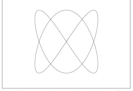
Fig. 6 – The Lissajous figure is the oldest of phase plane plots. The two sinewave frequencies shown here are in a ratio of 3:2.
