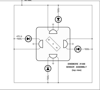
Fig. 5 – LOW END DIGITAL COMPASS is cheaper than a fluxgate but has a very poor resolution. Hall effect sensors are used to drive the LED outputs as shown here. Eight point LCD compass rose displays are also possible.
