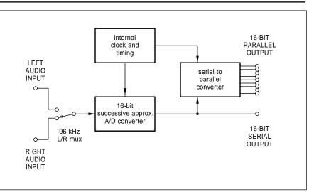
Fig. 2 – A SIMPLIFIED BLOCK DIAGRAM of the CDB5126 stereo audio A/D front end board. Because of a factory tested layout, nearly all of the usual black magic involving ground noise, shielding, and guarding has been done for you.
