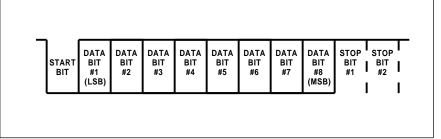
Fig. 3 – Most RS-232 serial communications will use this older "teletype" asynchronous code. Seven or eight data bits are normally used, with the least significant bit always sent first. Any number of stop bits above the minimum can be sent between successive characters.
