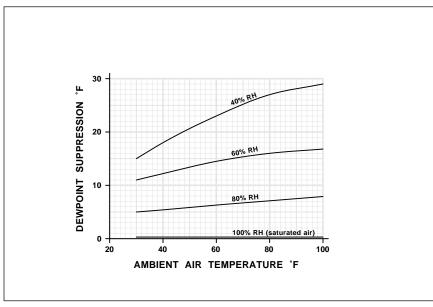
Fig. 3 – PRECISION LABORATORY MEASUREMENT of relative humidity is done by chilling the air to its dewpoint to find the equivalent air temperature for full saturation. Usually a servo driven mirror will fog or frost at the dewpoint, altering a sensing beam of light. Dewpoint measurements are best used at the higher humidity and temperature ranges.
