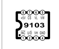
FIG. 2 – EEPOT Pinouts. VL, VW, and VH are the terminals for the output potentiometer. The CS chip select is brought low to change the wiper position, but is otherwise left at +5. The position gets changed by bringing TNC first low and then high again, with the direction set by the up-down pin U/D. A high on U/D will advance the position.
