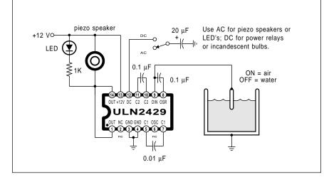
Fig. 3 – The Sprague ULN 2429 is an automotive liquid level detector that has plenty of hacker potential. Here is the basic test circuit using a pop can full of tap water as a liquid level sensor.
