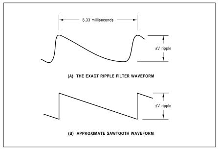
Fig. 2 – THE EXACT AND APPROXIMATE voltage waveforms as found across the ripple filter capacitor. Note that the diodes only conduct very briefly during the middle of each ac line half cycle.
