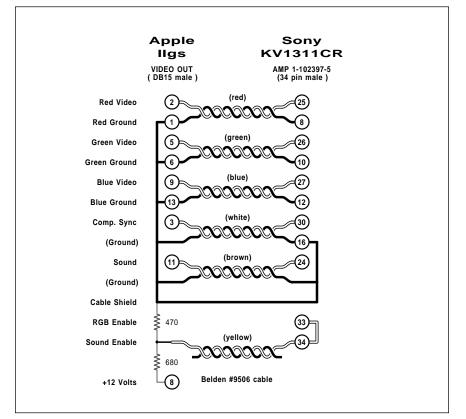
Fig. 2 – An interface cable to go between the Apple IIgs computer and the Sony KV-1311-CR linear RGB monitor/receiver.
