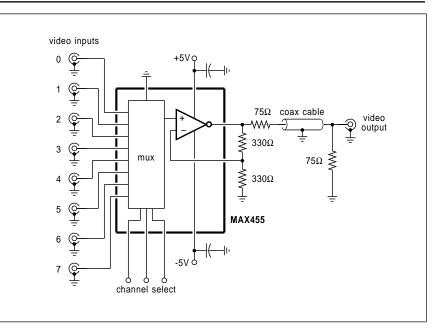
Fig. 3 – An eight position, single chip video selector and driver.
