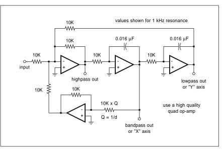
Fig. 4 – THIS STATE VARIABLE ACTIVE FILTER can give you lowpass, bandpass and highpass outputs, and is a good "workhorse" circuit for both low and high Q uses. This is also a handy test circuit for exploring phase plane plots on your own.
