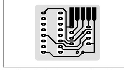
Fig. 6 – One possible pc layout for your converter. The ground plane on the component side is an absolute must! The view here is from the foil side.
