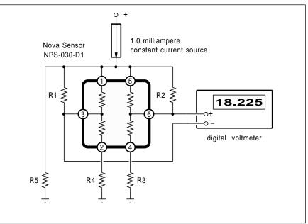
Fig. 5 – Extra resistors can be provided for temperature compensation and for span adjustments. Correct values are specified for each sensor.
