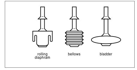
Fig. 2 – The formost rule of low pressure hacker pneumatics is this: NEVER have any seal that moves! Here are some actuator ideas to get you started.
