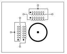
Fig. 2 – IN A UNIPOLAR (or bifilar) stepper motor, you will find a pair of windings for each pahse. While this raises the cost and also reduces the available stepper power, your driver circuitry is vastly simplier and very much cheaper, since only a current sink is needed for each winding. A unipolar stepper often has six leads.
