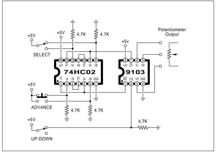
Fig. 3 – Use this circuit to test your EEPOT. The debouncing shown is only needed when you are using mechanical contacts.
