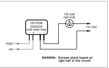
Fig. 2 – This simpler but more expensive ac power output computer interface needs only one part. Once again, a low logic input will light the lamp.
