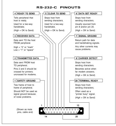
Fig. 1 – Here are some details on the RS-232 serial communications standard. Note that the data and handshake lines are often crossed for printers and uncrossed for modems.
