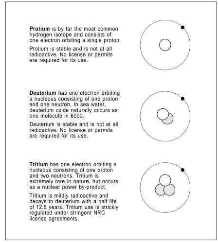
Fig. 2 – ISOTOPES are variations on an element that will have different atomic weights but largely identical chemical properties. The three isotopes of hydrogen are shown here. The Deuterium isotope gets used in the cold fusion experiments, initially in the form of deuterium oxide or "heavy water".
