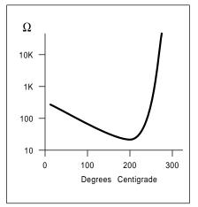
Fig. 1 – A typical resistance versus temperature curve for a posistor. If you exceed the critical temperature, the resistance sharply increases and the current dramatically drops.
