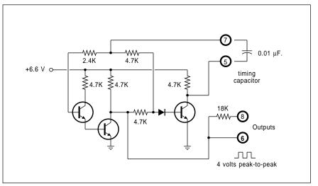
Fig. 4 – A simplified schematic of the internal audio oscillator found in the ULN 2429. The usual operating frequncy is 2.5 kiloHertz, and can be set by the external timing capacitor.
