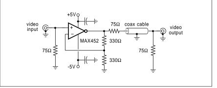
Fig. 4 – The video driver is separately available as the MAX452.
