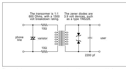
Fig. 2 – A data access arrangement such as this one must provide for surge suppression, signal limiting and safety isolation, as well as being FCC part 68 type approved.
