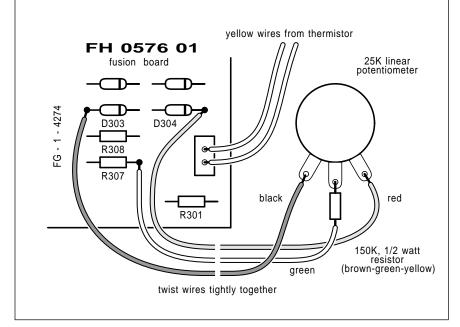
Fig. 6 – The pictorial diagram for the Canon fuser unit modification. The mod costs around 60 cents and can be done in twenty minutes.
