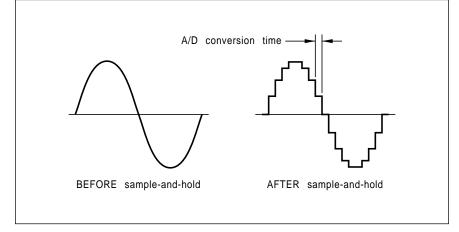
Fig. 3 - A sample and hold is needed to hold the analog input signal constant during the conversion time, or serious errors are certain to result.
