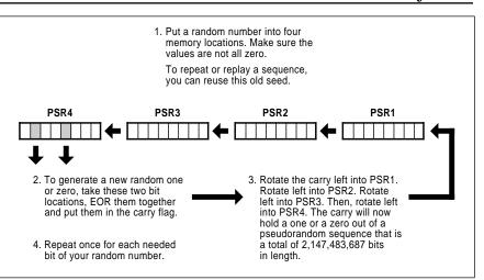
Fig. 3 - A 31 stage pseudorandom sequence generator done in software will produce a "random" string of 2,147,483,687 ones or zeros before it will start to exactly repeat. Typical execution time is under 40 microseconds.
