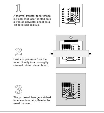
Fig. 3 – OUR NEW DIRECT TONER TRANSFER method can dramatically simplify and speed up making all of your hacker printed circuits at costs of only pennies per board. The process takes around twenty seconds.
