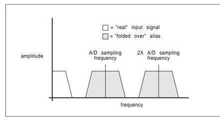
Fig. 2 – An anti-aliasing filter absolutely must be used with any A/D converter so as to sharply reject any and all frequencies above one-half of the sampling frequency. Should any higher frequencies remain present, they will "fold over" and form aliases that end up looking just like "real" input signals.
