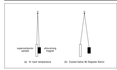
Fig. 2 – The Meissner Effect will produce a zero internal magnetic field in a cooled superconductor. The resulting field distortion will deflect (or can even levitate!) an extremely strong magnet as shown.
