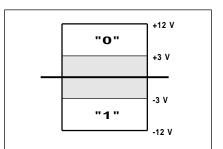
Fig. 2 – Here are the two logic levels that are normally needed for RS-232 communications. A "negative logic" convention is always used.
