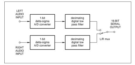
Fig. 7 – A SIMPLIFIED BLOCK DIAGRAM of the CSZ5326 A/D. The mind blowing specs here do include a 95 decibel dynamic range, 106 decibels of signal/noise ratio, 0.001 decibels of passband ripple, and a 0.0015 percent harmonic distortion for both 44 kHz stereo channels.
