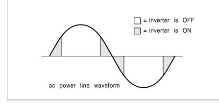
Fig. 6 - A syncrhronous inverter can be used to feed surplus energy from a solar panel or other alternate energy source back into the power line. Here is one possible waveform.
