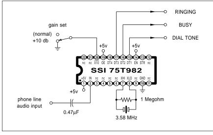
Fig. 2 – A CIRCUIT TO DETECT the "new" or "precise" call progress signals. This is a Silicon Systems chip; others are available from Signetics or Teltone.
