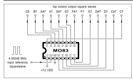
Fig. 5 – A top octave generator integrated circuit takes an input reference square wave and divides it down to approximate the thirteen uppermost notes on an electronic organ. Further binary division of each output can generate all the needed lower notes. This SGS part replaces the Mostek MK5083.
