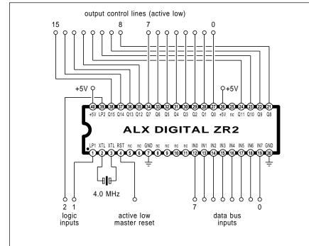
Fig. 5 – THE ZR2 "DISCO CHIP" is programmable to handle many light chasers, zoners, and ac/dc dimmers, along with other communications, counting, and control tasks. It is based on a programmable peripheral interface chip from Intel.
