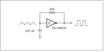
Fig. 1 – AN ELEGANTLY SIMPLE oscillator can be built using nothing but one resistor, a capacitor, and 1/6th of a CMOS hex Schmitt Trigger. Your output is a full supply square wave, while the input is a triangular wave that "saws" between the trigger's upper and lower trip points.
