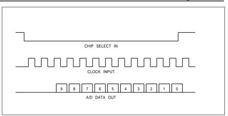
Fig. 4 – The timing waveforms used with the LTC1092. Your computer or other external timing inputs a chip select and thirteen clock pulses. Then, the LTC1092 responds in turn with ten A/D serial data bits. The A/D conversion speed can be as fast as 45 kHz.
