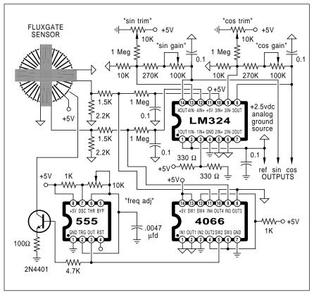
Fig. 4 - A simplified schematic of a solid state digital compass. The outputs are A/D converted and then routed to a microprocessor that handles the bearing calculations and a suitable digital display.
