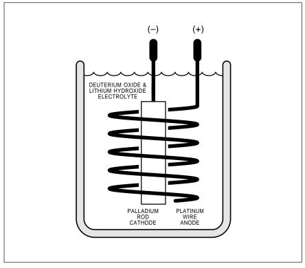
Fig. 4 – COLD FUSION appears to get produced in this experimental electrolytic cell. The heavy water dissociates into deuterium and oxygen ions. The deuterium ions will migrate to the palladium cathode where many of them become trapped in its crystalline structure. Some of the later arriving deuterium ions apparently cold fuse with the trapped ones, apparently producing both heat and at least a few of the expected fusion by-products. But it is far too soon to tell for sure.
