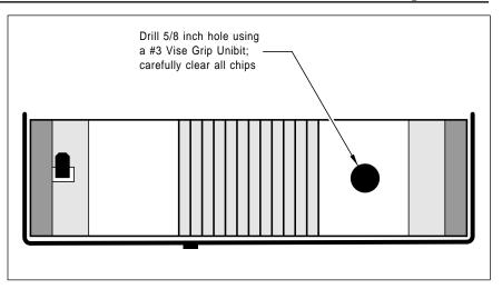
Fig. 3 – Adding a fresh toner filling hole to a SX cartridge.
