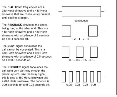
Fig. 1 – TELEPHONE CALL PROGRESS signals can be detected by both their frequency and their cadence. Here are all the US standards for the "precise" or the "new" call progress tones.
