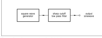
Fig. 1 – Brute force generation of a digital sinewave creates a square wave and then sharply low pass filters it. Triangular or certain "magic" waveforms can give you much better results than a square wave.
