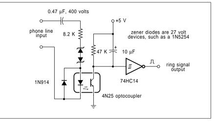
Fig. 4 – A telephone ring detector. The optocoupler provides safety isolation, while the capacitor converts the individual rings into a continuous signal.
