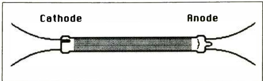
Fig. 3. The JKL BF659 lamp is only 2½" long and comes in several colors. It is very easy to power, from the ac line or transistor oscillator. Take careful note of polarity.
