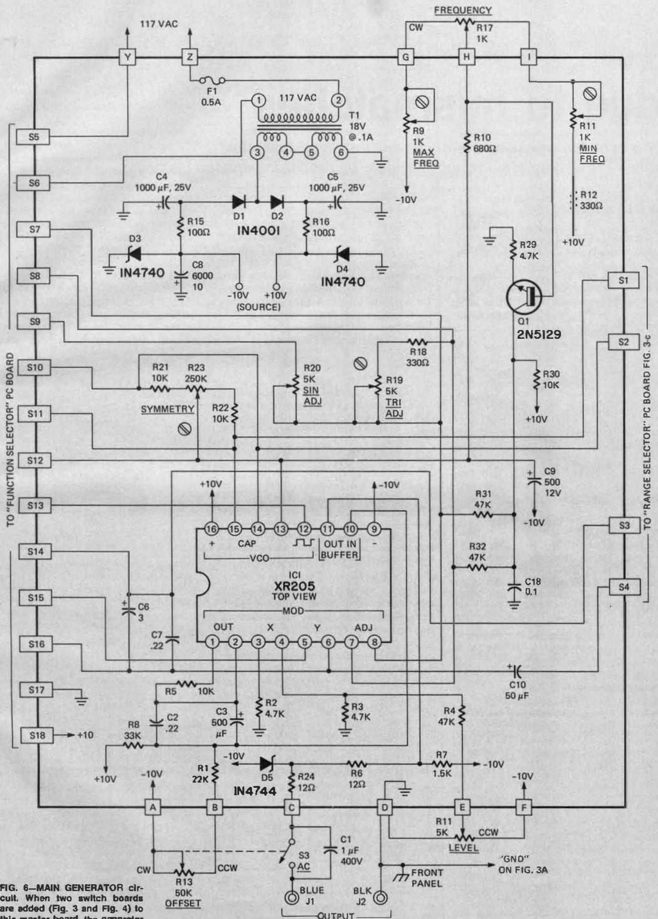
FIG. 6—MAIN GENERATOR circuit. When two switch boards are added (Fig. 3 and Fig. 4) to this master board, the generator is complete.
