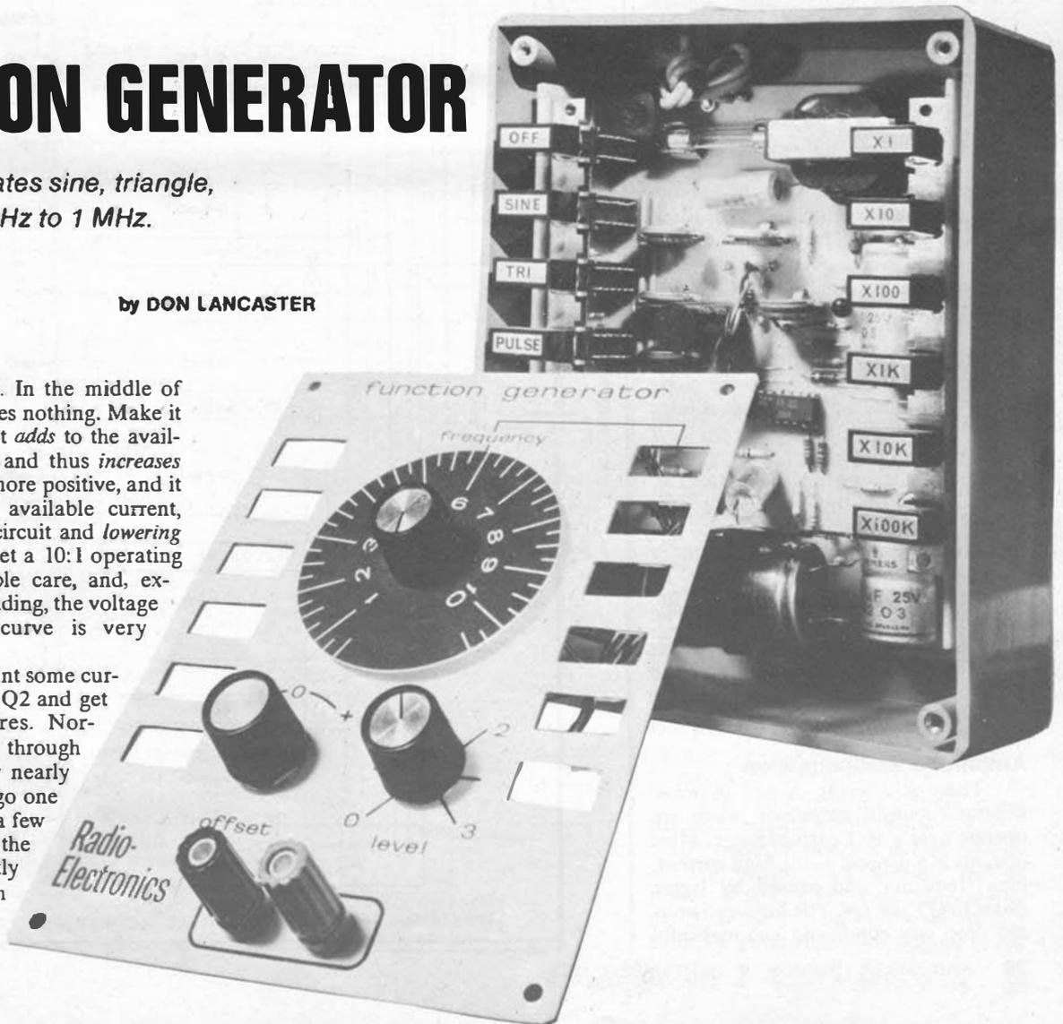
does is knock the sharp corners off the triangle waveshape, giving us the familiar sinewave shape, with a distortion typically around 2%. This technique is far simpler than those normally used in function generators, and this level of distortion is not even noticeable for anything but critical audio testing.
