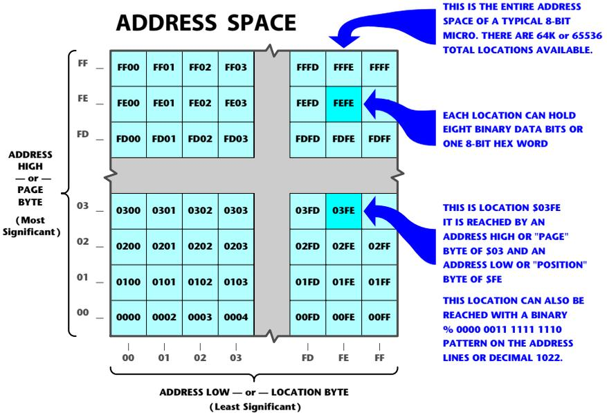
We see that we have 65536 boxes and that these boxes are numbered in order from hex \$0000 through \$FFFF. Besides finding a box by its number, we could also locate any box by finding its row and column instead.
