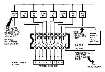
This octal peripheral driver comes in an 18-pin package and handles eight separate loads of up to half an ampere each, powered from an outside supply of 40 volts or less. The inside circuitry consists of eight separate Darlington transistor drivers, along with eight separate spike-protecting diodes. Once again, this supply *must* share a common ground with the microcomputer and the peripheral chip.
