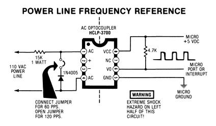
This special *Hewlett Packard* AC optocoupler directly and safely accepts a full strengh 110-volt AC line signal at its inputs by way of a large current-limiting resistor. This lights one or the other of the input LEDs, except during line zero crossings. The output of the optocoupler will go positive on each zero crossing of the AC line, giving you 120 pulses per second into your port. Extra goodies inside the chip improve the snap-action and stability.
