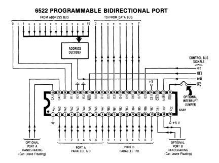
The port lines are arranged by eights into an A port and a B port. The supply power and system bus pins are connected the usual way. Four optional input or output lines intended for handshaking are called CA1, CA2, CB1, and CB2. These may be left unconnected for simple I/O uses.
