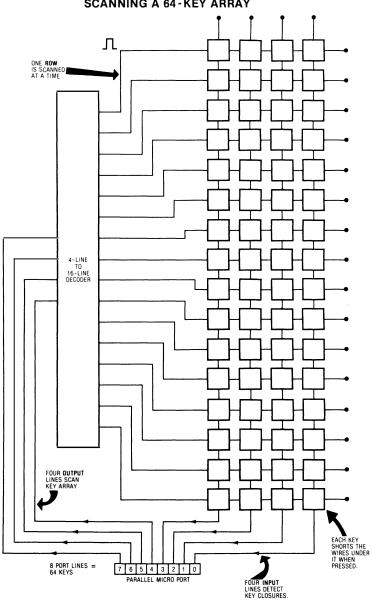
We see that we can get by with only eight lines from a single bidirectional I/O port to handle all sixty-four keys.
