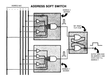
Here we have two decoders set to two different addresses. Address X sets a set-reset flip-flop and drives the output high. Address Y clears the set-reset flip-flop and drives the output low. The output stays low till address X is hit and then stays high till address Y is flashed.
