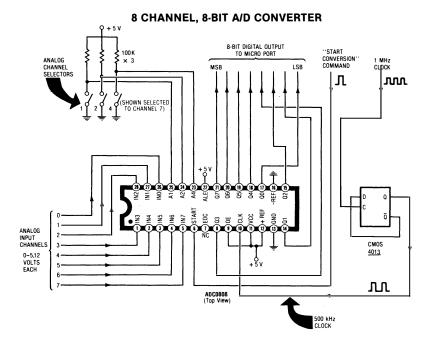
This has to be one of the cheapest, simplest, and easiest to use A/D converters anywhere. *National* builds it using CMOS technology, with several second sources. You simply hang the chip onto some port lines, apply a single +5-volt power supply, add a clock, and away it goes.
