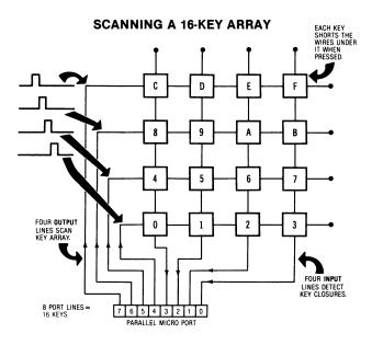
We use four output port lines and four input port lines. Only a single output line is allowed to go high at any instant. The output lines take turns going round and round as shown.
