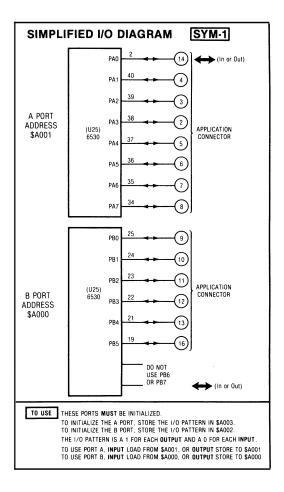
This time, we have only fourteen I/O lines immediately available, and they come from a single IC, a 6530 called U25. The 6530 is a fancy upgrade of the 6522. All of the lines appear at the "Application" connector on the pins that are numbered as shown.
