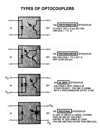
Most optocoupler use an LED as a light source. These are easily driven by most micro ports. Infrared light is used since its spectrum is more compatible with many light sensors and since you won't be watching it anyway. Almost all optocouplers are opaque packaged so that room lighting has no effect. As with any LED, you must be careful of the circuit polarity and must limit input current to a safe value, typically 10 milliamperes.
