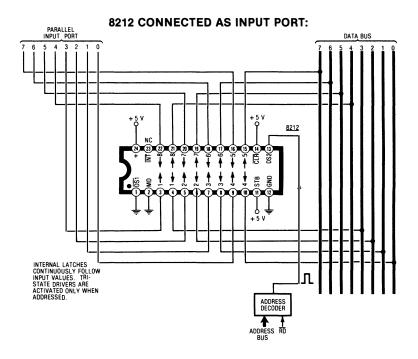
The eight parallel port lines are wired to the inputs of the eight storage latches, and the eight tri-state driver outputs go to the data bus. Note that the mode input on pin two is grounded.
