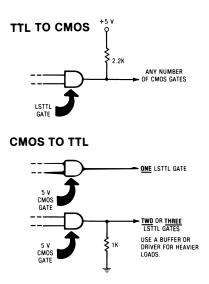
The pulldown resistor in the CMOS to LSTTL interface is only needed if you are driving two or three LSTTL inputs from one CMOS output. This same circuit can be used to drive one old-fashioned regular TTL input.
