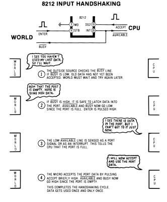
The "port is full" flip-flop outputs on the  $\overline{INT}$  line of pin 23. This pin is active low, meaning that a high signal here equals an empty port. For input, the  $\overline{INT}$  pin goes to the CPU as an AVAILABLE signal and goes to the outside world as a  $\overline{BUSY}$  signal.
