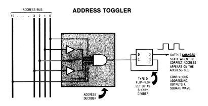
When you address the magic location, the output changes state. Address the location again, and the output changes once more, going from zero to one or vice versa. To output a square wave, you continuously address the magic location at *twice* the output frequency you want . . .
