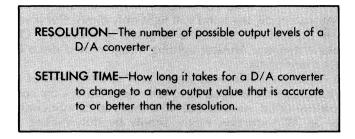
For instance, an 8-bit D/A converter would have 256 possible analog output levels and thus would be accurate to something like one-half percent. A 12-bit D/A converter would have 4096 possible analog output levels and thus would be accurate to one part in 4096 or around .025 percent.
