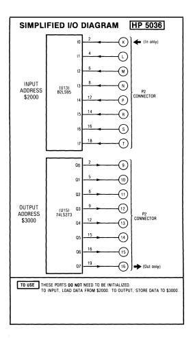
On this trainer, we have 8 input lines on top and 8 output lines at the bottom, both accessed via connector P2. Looking more closely, we see that input I0 ("EYE-ZERO") enters the trainer via pin K of P2, and so on down the list.
