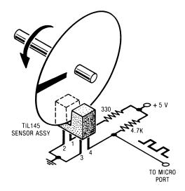
What I have done here is to take an interrupting optocoupler pair and interpose a disk with clear and opaque sectors on it. Depending on your use, this can be a tachometer or a position sensor, and it can be used for anything from an anemometer to a trackball to a robotic position sensor to a miles-per-gallon meter.
