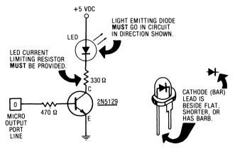
As before, a port high provides base current which saturates the transistor and lights the LED. A port low stops base current which turns off the transistor and puts out the LED.
