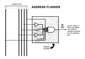
What you do is decode the address bus to a unique state or group of states. Anytime you hit one of the magic addresses, the output of the decoder briefly goes high and can be used to control something. That something can be a line to the outside world or anything inside the system that needs a brief pulse to attract its attention, such as a handshaking reset or a strobe.
