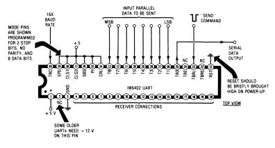
First you supply this 40-pin chip by putting +5 on pin 1 and grounding pin 3. This *Intersil* 6402 is a modern, single supply chip. Older devices may also want a -12-volt supply on pin 2.
