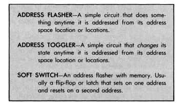
An important advantage of these "less than a port" output schemes is that they do not have to get involved with the data bus or any of the working registers of a micro. Thus, you can get a single-bit output through any of these without changing anything important in your microcomputer. This output can go to the outside world or be used to change the operating mode of your micro.
