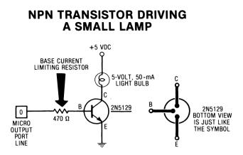
In this case, the lamp is the load for our NPN transistor. If the micro port provides a weak high output, this output in turn gives us transistor base current, turns the transistor on and saturates it, and puts nearly the full supply voltage across the lamp. This, of course, lights the bulb.
