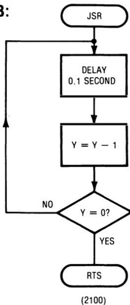
All we have to do here is rip off the code for the 0.1-second delay and remove the bottom RTS. Then we decrement Y, test Y for zero, and repeat the 0.1-second delay Y times. When Y hits zero, we finally return. The number of tenths of a second delay you get is set by the number you put into the Y register, which in turn sets the number of trips through the “.1” code.
