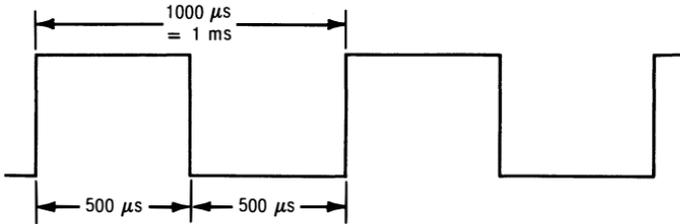
This square wave has a frequency of 1 kilohertz and a period of 1 millisecond. It is high for half a millisecond, or 500 microseconds, and low for another 500 microseconds.
