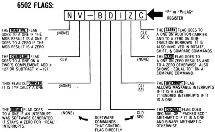
Starting at the left, we have our N, or negative, flag which sets on an MSB one and clears on an MSB zero and is typical of most any micro.
