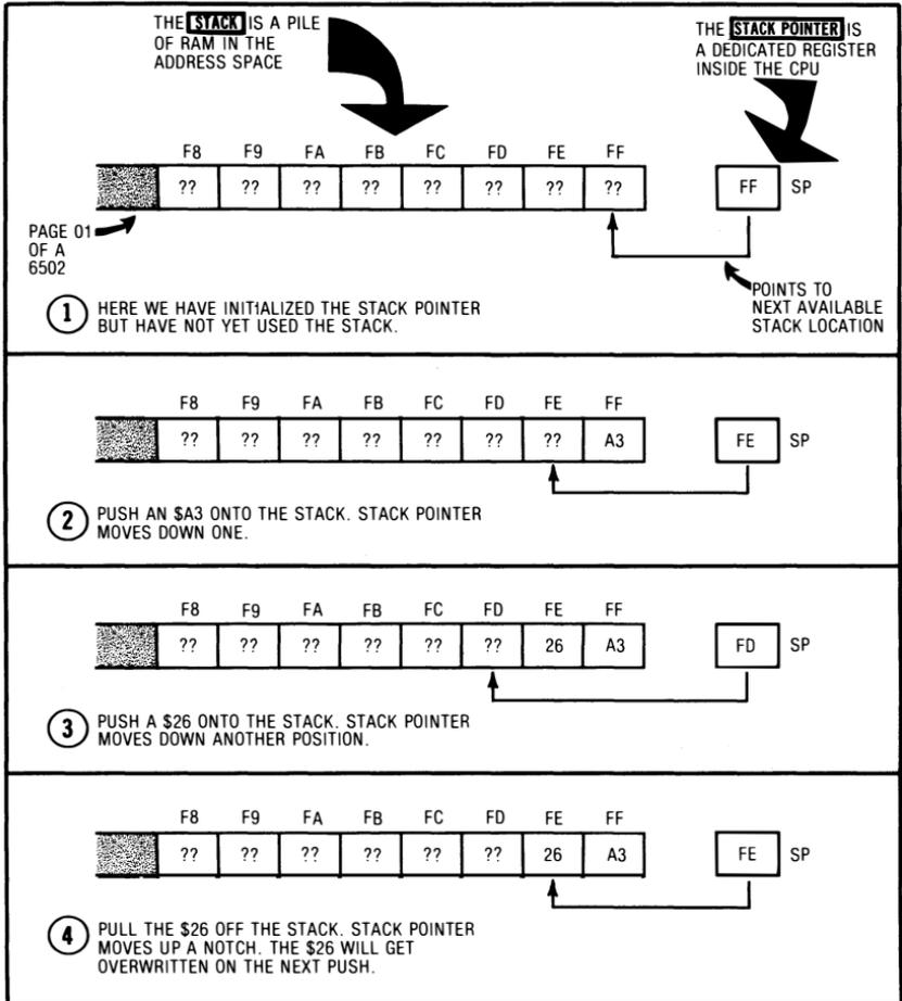
Remember that the stack is a bunch of cleverly disguised RAM on page one, while the stack pointer is an 8-bit dedicated use register inside the CPU. You initialize the stack pointer to \$FF, which becomes \$01FF when the CPU gets done playing with it. As you push things onto the stack, the stack pointer decrements itself to \$FE, \$FD, and so on down. As you pull things off the stack, the stack pointer increments itself to \$FD, \$FE, \$FF, and so on up.
