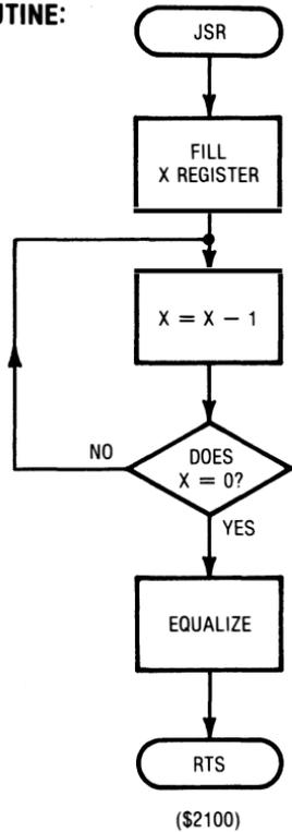
Note that our flowchart is now in two pieces. We have the high level flowchart that includes a box called "STALL VIA SUB." And we have the low level flowchart that gives us full details on how we
