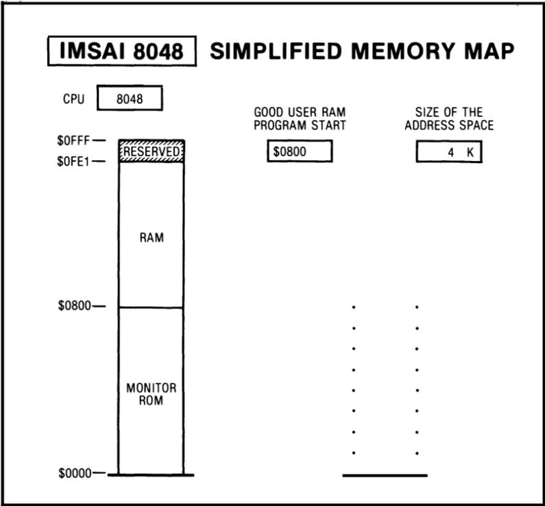
This trainer is extinct, but it does show us the typical layout for most current 8048 microcomputers. The 8048 is a smaller microprocessor intended for dedicated control uses. Its normal memory map is only 4K, or one-sixteenth the size of the two we just looked at. This memory space is split into two *banks* of 2K each. The ROM
