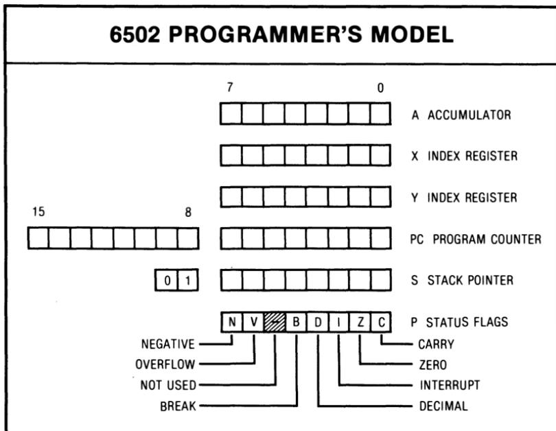
We see at once that the 6502 school has fewer and shorter working registers than the 8085. There is an 8-bit general-use accumulator and a pair of intended-use 8-bit X and Y registers. There is a 16-bit wide program counter that can point anywhere in the address
