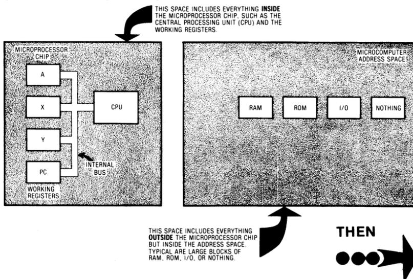
We see that we have a block called a microprocessor. This microprocessor contains a CPU, short for Central Processing Unit. The CPU acts as a postmaster to control totally what goes on where in the system. The CPU has immediate control over a group of working registers. How many of what kind depends on the micro you have chosen and is shown by the upcoming programmer's model.
