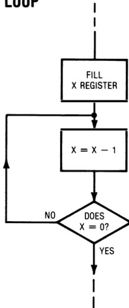
What you do is fill a register with a value and then knock one off that value over and over again until you reach zero. The net result is a long time delay that reuses the loop instructions over and over again as long as needed.
