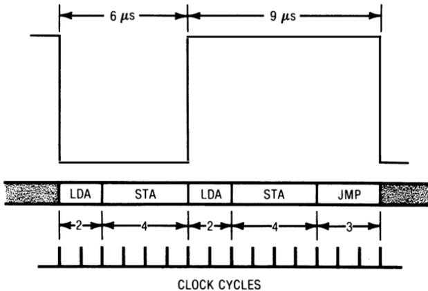
We can make our rectangular wave into a square wave by adding another 3 microseconds of delay during the time the output is low. We might try using a NOP, but this gives us only 2 microseconds of extra delay. Two NOPs together will overdo it and give us 4 microseconds of extra delay.
