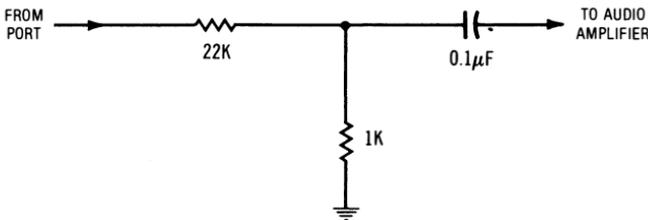
The reason for this “listener” probe is to knock the 5-volt square wave down to something that won’t overload the sensitive input of your usual audio amplifier. The tone should, of course, be there only when the program is running. Try stopping and starting the program to verify that you are actually generating the tone with your software.
