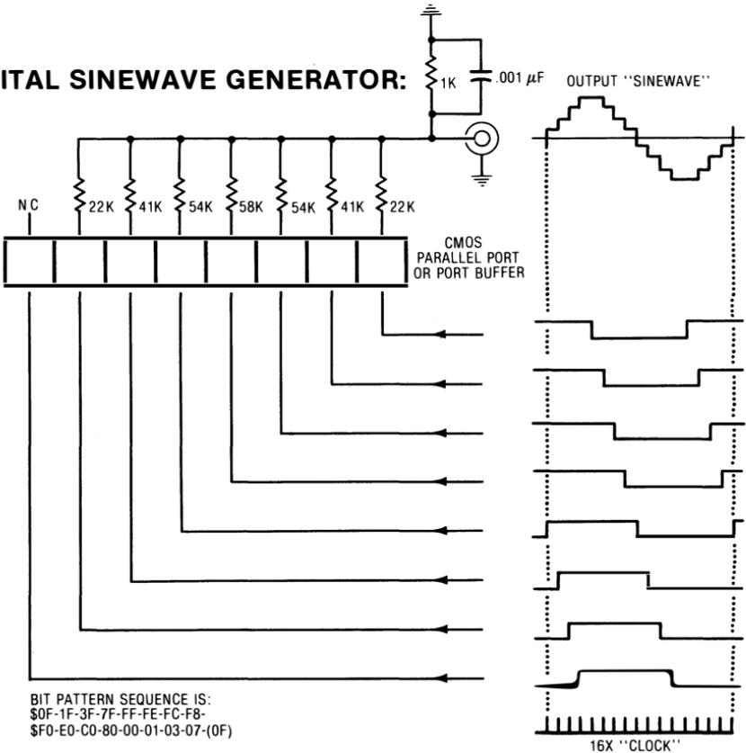
What you do is take all eight port lines and provide just the right pattern in just the right way to synthesize a good sinewave. This particular one will have its first two "loud" harmonics as the fifteenth at 1/15 amplitude and the seventeenth at 1/17 amplitude,
