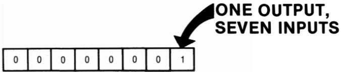
. . . which in this case is a hex \$01. So we write this pattern to our teaching location \$C080 by first filling the accumulator immediately with the value \$01 and then by storing the accumulator into the teaching location.
