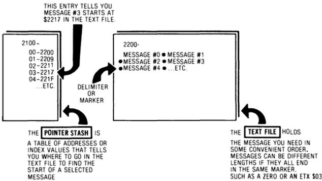
Each message ends with a *marker* or *delimiter* of some sort, such as a 00 NUL or an ASCII “End of Text” ETX or \$03 command . . .
