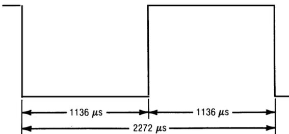
The exact time period of a 440-hertz square wave is 2272.72 microseconds, or 1136.36 clock cycles per half cycle. But the closest we can hit this is 1136 cycles on a trainer with a 1-microsecond CPU cycle time. Is this accurate enough?
