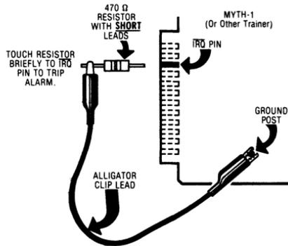
What you do is ground the  $\overline{\text{IRQ}}$  pin on the trainer’s I/O connector through a small resistor. Briefly touching the resistor to the  $\overline{\text{IRQ}}$  pin should trip the alarm.
