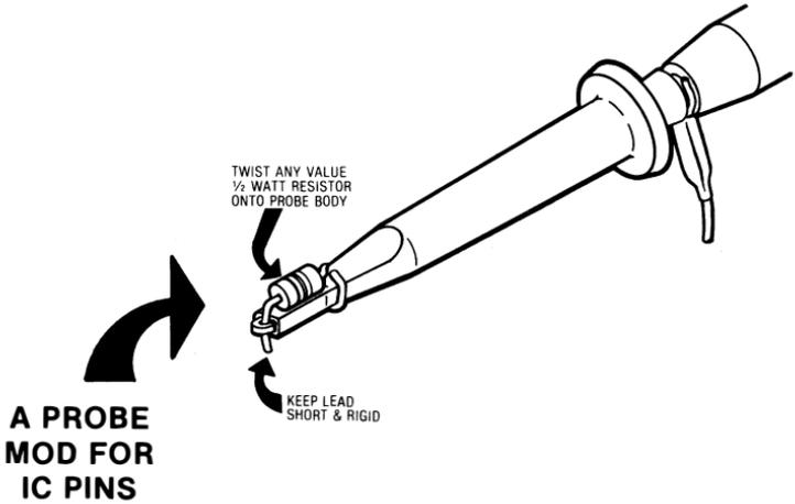
Any old value half-watt resistor will work. Be sure the lead is just long enough to give you a convenient and rigid way to touch a single integrated circuit pin. Some probe accessory kits may have screw-on pin probe attachments. Use whatever you have available. A gotcha . . .
