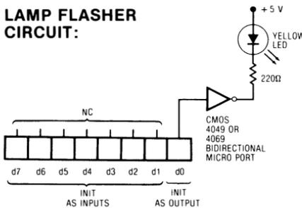
Our main program is only slightly longer than the earlier delay programs. We use a .Y-second delay subroutine, but we have to pass Y a value from the main program before we go to the .Y-second delay subroutine.
