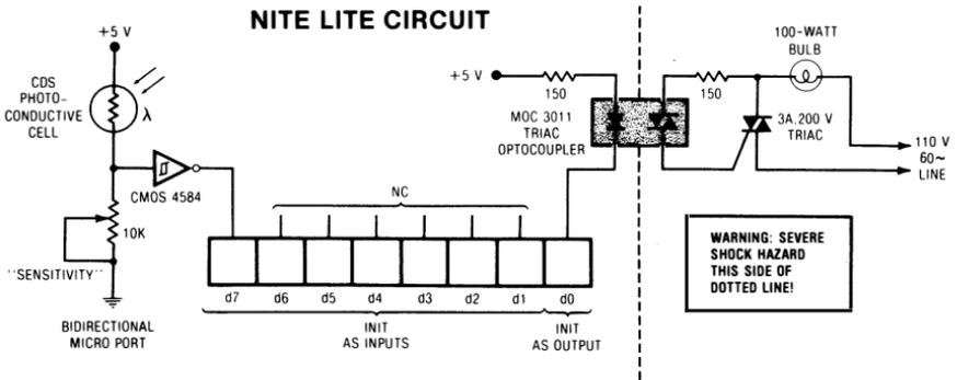
We route the output of the photocell circuit into an input on one bit line of a single port. We route the output of the microcomputer to an output bit line of a port. We'll assume you have a bidirectional I/O port, and that you will input on the MSB line B7 and output on the LSB line B0 of the same port of our MYTH-1 trainer.
