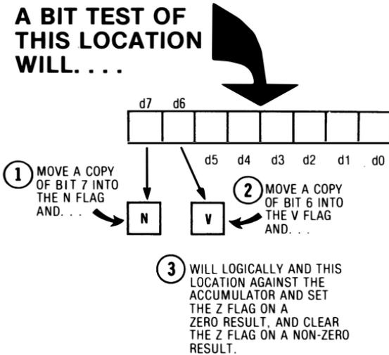
In this first way to use the BIT test, everything happens free and automatically. You don't have to worry about what is in the accumulator. Since only bits 6 and 7 get moved into the flags, though, it always pays to put the things to be tested on the highest two bits of any word . . .
