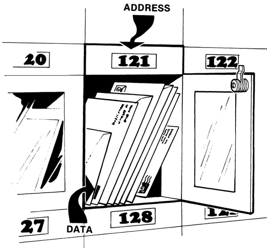
Once again, an address is a location, and data is what goes in that location. Each address in a microcomputer must be unique. No mix-ups can be allowed. The addresses in the address space are often identified by a hex number. The working registers are usually identified by name or by a single letter.
