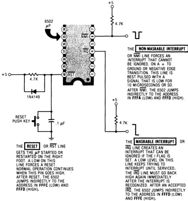
The resistor and capacitor on the RST line gives you an automatic reset interrupt on power-up. When you first apply power, the capacitor is slow to charge, and the system is held reset until the RST line goes high enough to release the interrupt. At that point, the computer starts off on a normal program. Should supply power be removed, the capacitor quickly discharges through the diode so it is ready to go on a fresh restart.
