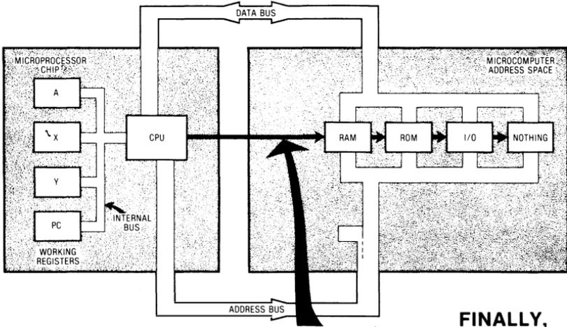
THE **CONTROL BUS** IS A GROUP OF WIRES THAT DECIDES READING VS. WRITING, SYNCHRONIZES TIMING, PROVIDES FOR INTERRUPTS AND RESETS, AND DOES OTHER HOUSEKEEPING CHORES.
