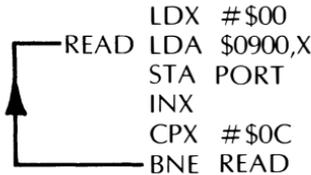
Well, even if it looks like gibberish, it is obviously much shorter gibberish than before. Let's see. First we load the X register with a zero value, and then load the accumulator with what is at \$0900 plus zero, or simply the contents of address \$0900. We then shove this out the port.
