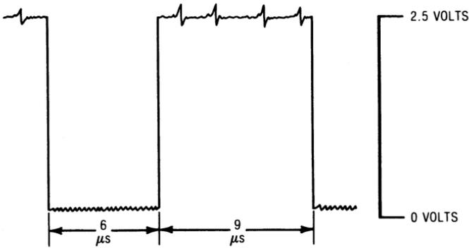
Uh, oops. That's a waveform all right, and the waveform comes and goes with running and not running of the program. But this is *not* a square wave. It is a *rectangular* one! The low time is clearly less than the high time.
