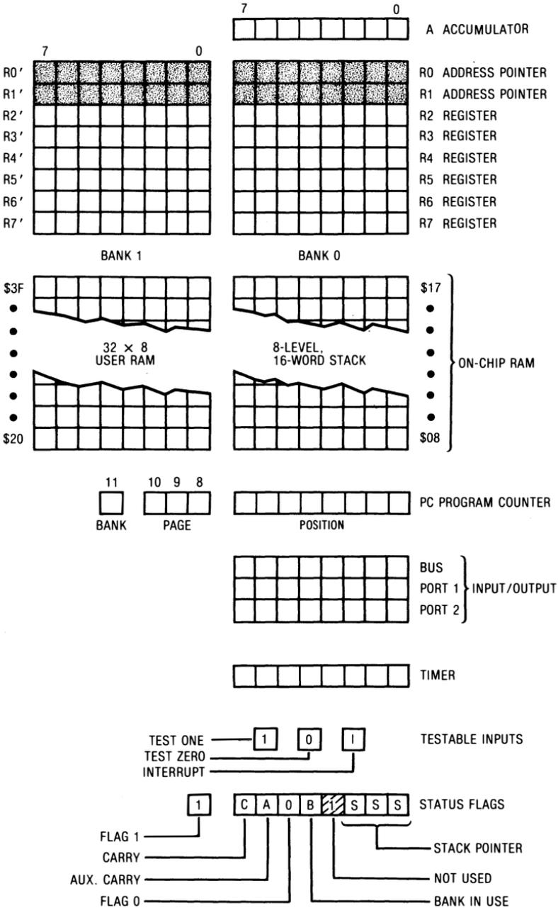
We see there is the usual 8-bit accumulator. In addition, there are sixteen working registers, numbered R0 through R7 and R0' through R7'. R0, R1, R0', and R1' are intended-use registers since they can contain an address for us. The others are general-use registers.
