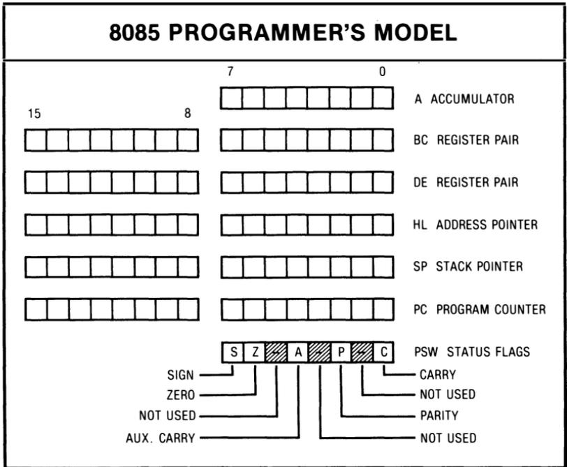
Each block corresponds to a single bit location. Each row of blocks corresponds to one working register. We see at the top that we have an accumulator that is eight bits wide. The accumulator usually ends up holding the result of a logic or arithmetic instruction.
