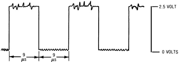
On other micro families, you may get holes chopped in the square wave or have other problems. Check the address bus at a memory chip pin or an expansion connector pin, rather than at the microprocessor chip, and see if it gets any better.
