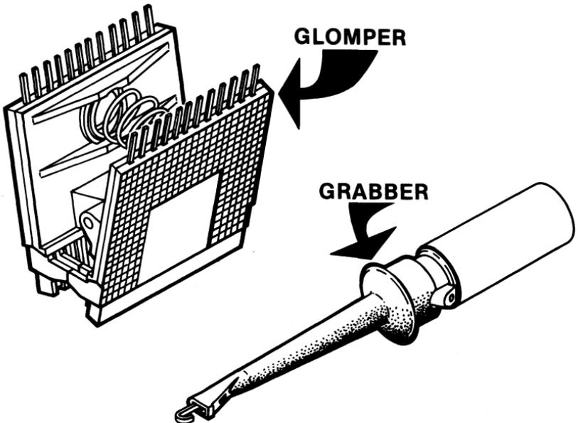
Glomper clips snap onto an integrated circuit and bring out all the pins to where you can conveniently reach them for measurement or scope viewing. Grabbers are tiny hook clips that let you
