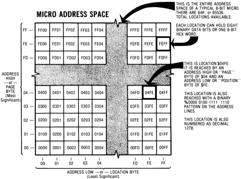
We see that we have 65536 boxes and that these boxes are numbered in order from hex \$0000 through \$FFFF. Besides finding a box by its number, we can also locate any box by finding its row and column.
