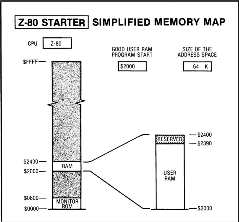
Since the Z-80 starter is from the 8080 school, we expect to find ROM on the bottom and RAM further up. In this case, our monitor takes up the first 2048 locations in the address space. This time, the reset and interrupt vectors go at the very bottom.
