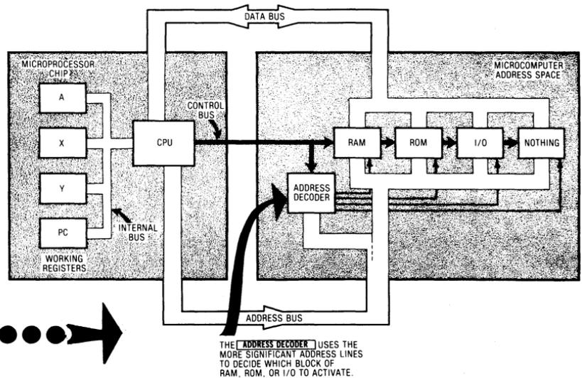
Reviewing, we see that the typical microcomputer has an internal microprocessor area and an external address space area, and that the two are normally separate. The microprocessor includes the CPU, which acts as postmaster or system traffic cop, along with some working registers that get involved as temporary stashes with just about everything the microcomputer does:
