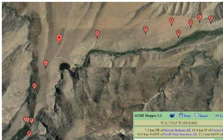
The Frye Complex portion of the canal delivery system is approximately 3 miles or 5 kilometers long with elevations ranging from 5800 down to 4200 feet, but not counting the selectable routing continuances of the **Robinson Canal**, or of the **Allen Canal**, and the **HS Canal**. These required slopes are far in excess of typical individual single canals lower in the hanging **bajada** canals system.
